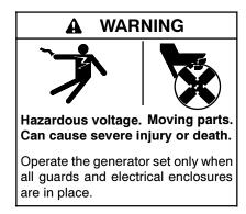
Servicing the generator set when it is operating. Exposed moving parts can cause severe injury or death. Keep hands, feet, hair, clothing, and test leads away from the belts and pulleys when the generator set is running. Replace guards, screens, and covers before operating the generator set
