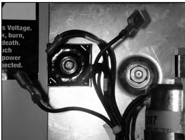
Figure 6-14 Rectifier Connections (DC solenoid leads shown disconnected)
