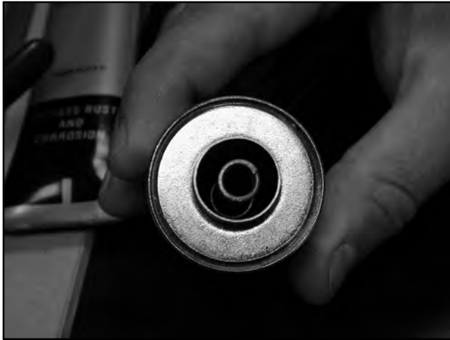
Figure 6-19 Spring Holder in Coil
