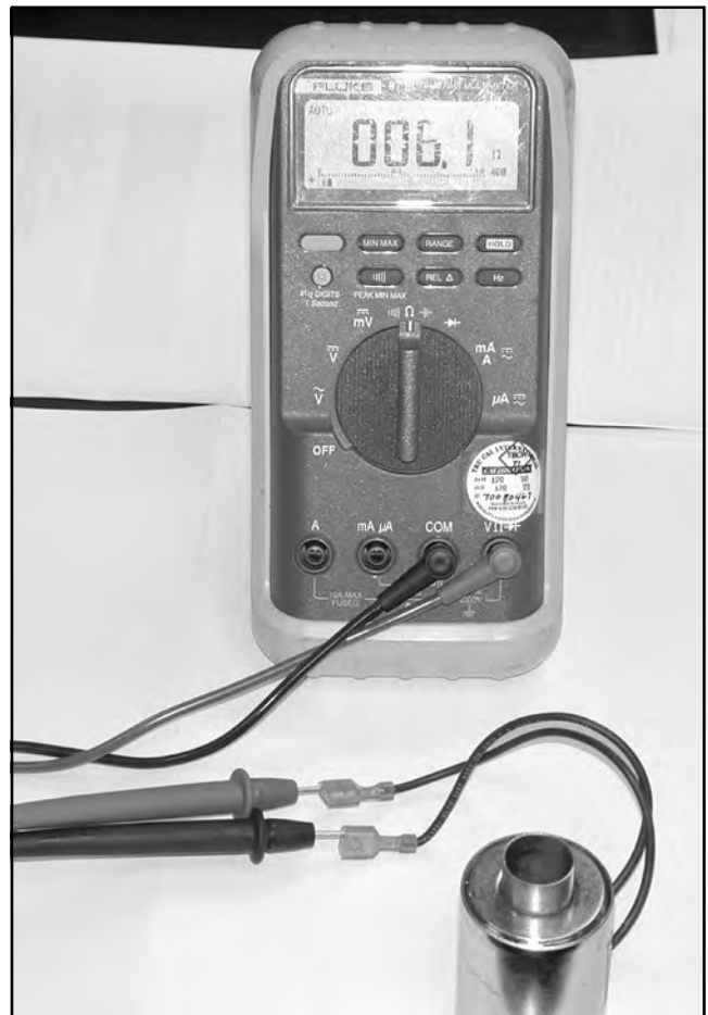
Figure 6-15 Checking Coil Resistance
