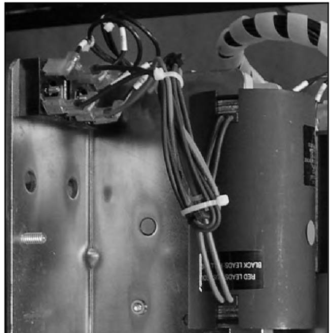
Figure 6-23 Rectifier Connections and Tie Wraps
