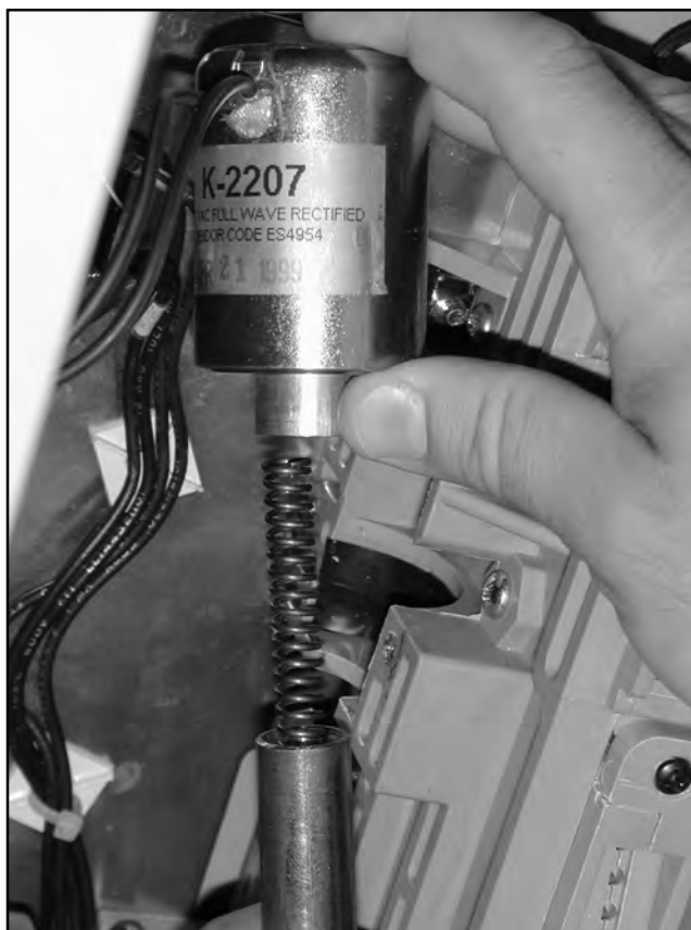
Figure 6-18 Spring and Plunger Assembly
