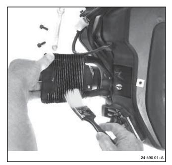
Figure 3-3 Cleaning Oil Cooler
