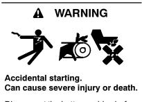
Disconnect the battery cables before working on the generator set. Remove the negative (-) lead first when disconnecting the battery. Reconnect the negative (-) lead last when reconnecting the battery.
