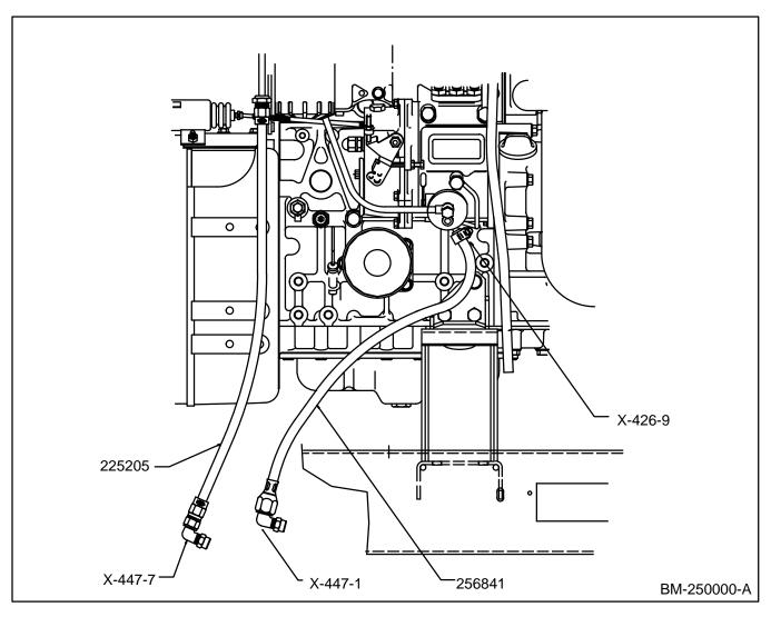
Figure 1. Flexible Fuel Line Connection 6 kW Diesel Standby Generators
