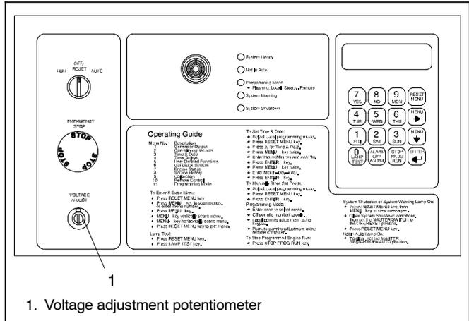
**Figure 3** Voltage Adjustment
