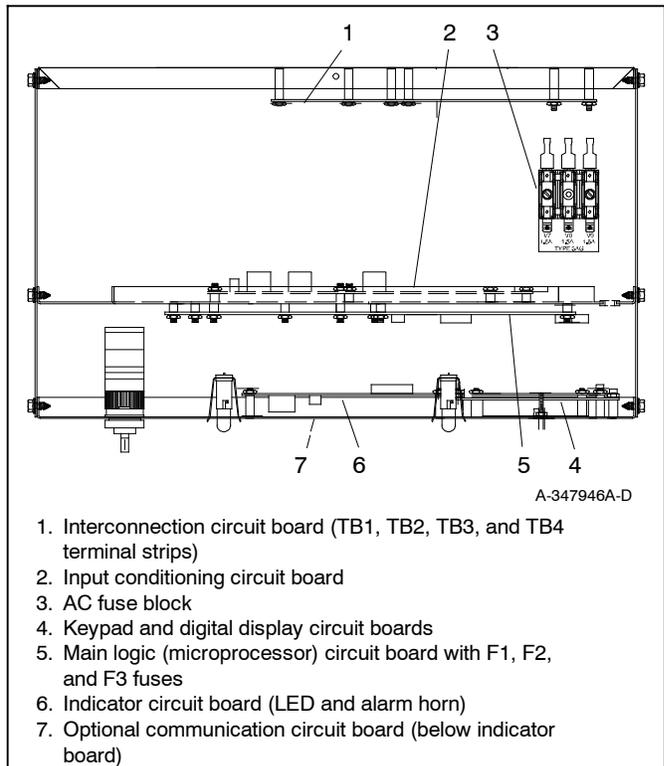
**Figure 4** Controller Circuit Boards and Fuses (controller top view)
