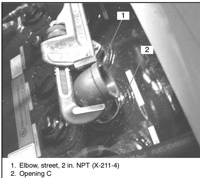
Figure 12 Secure Subassembly into Opening C
