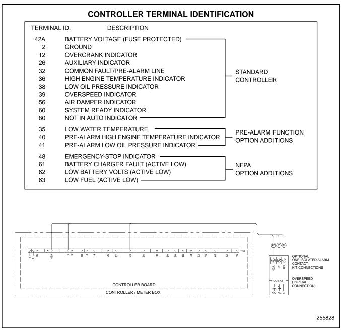
Figure 2. Wiring Diagram
