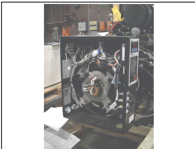
Figure 9 Junction Box Shown with Cover Removed
