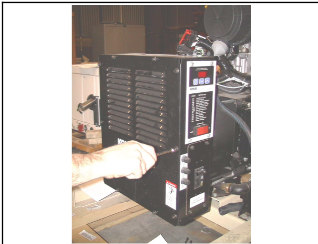
Figure 8 Junction Box Cover Screws
