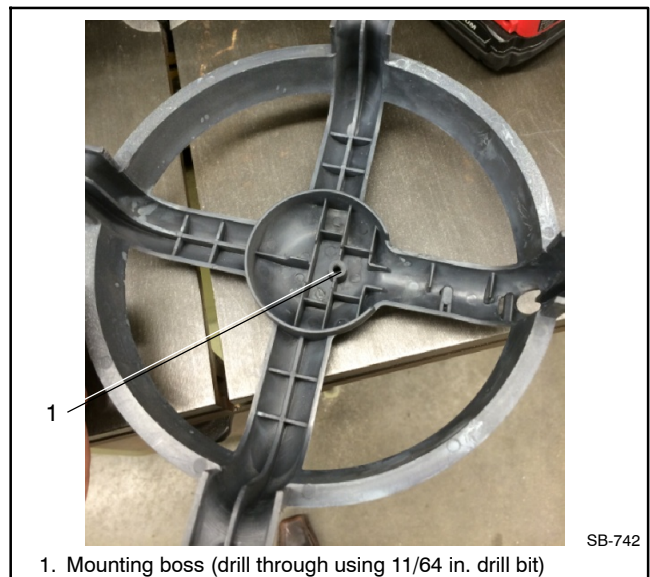
Figure 4 Drill Hole Through Mounting Boss
