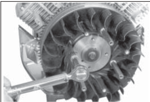
Figure 11-33. Torquing Supports for Metal Screen (Some Models).
