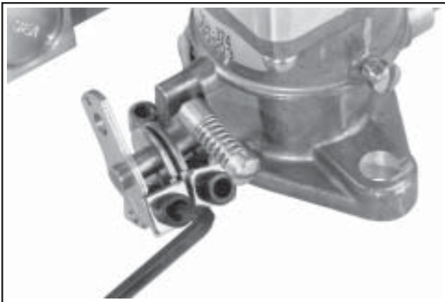
Figure 5A-14. Tightening Throttle Linkage Clamp Bracket.
