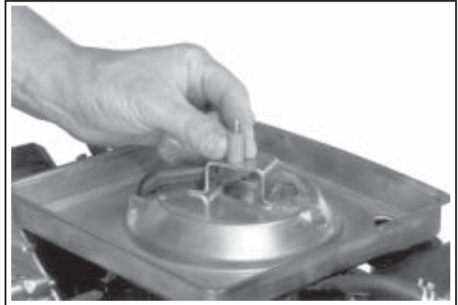
Figure 9-8. Removing Air Cleaner Base Retainer.
