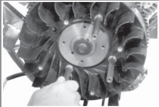
Figure 11-32. Installing Supports for Metal Grass Screen.
