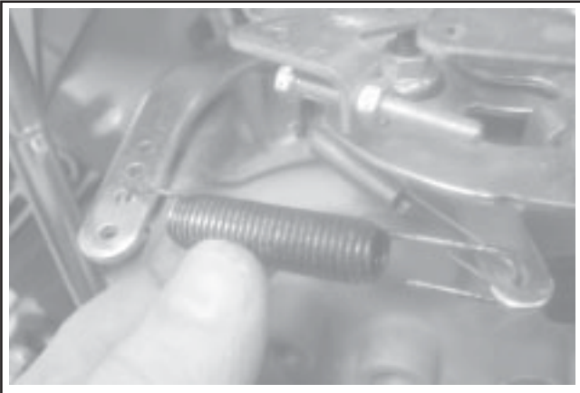
Figure 11-85. Connecting Spring to Governor Lever.
