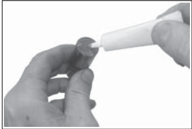
Figure 11-34. Applying Camshaft Lubricant to Bottom of Lifters.
