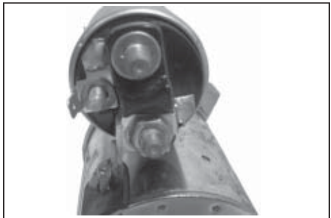
Figure 8-73. Positive (+) Brush Lead Connection.
