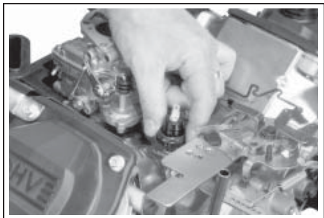
Figure 11-88. Installing Oil Sentry™ Switch.
