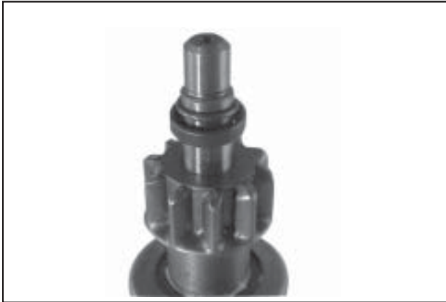
Figure 8-53. Retaining Ring Detail.
