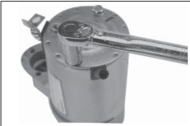
Figure 8-71. Torquing Thru Bolts.
