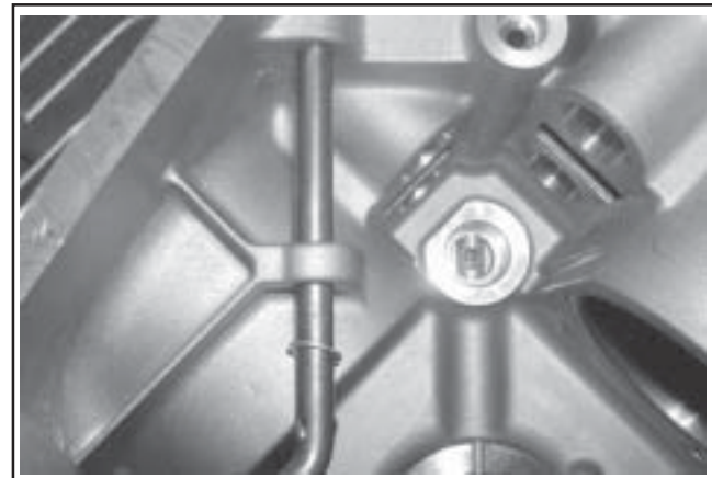
Figure 11-5. Installing 8 mm Governor Cross Shaft.
