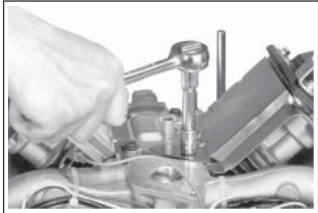
Figure 9-39. Removing Fasteners Holding Baffle and Breather Cover.
