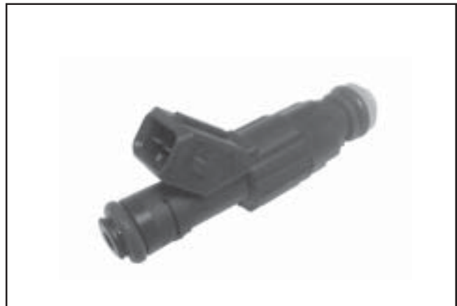
Figure 5B-17. Style 2 Fuel Injector.
