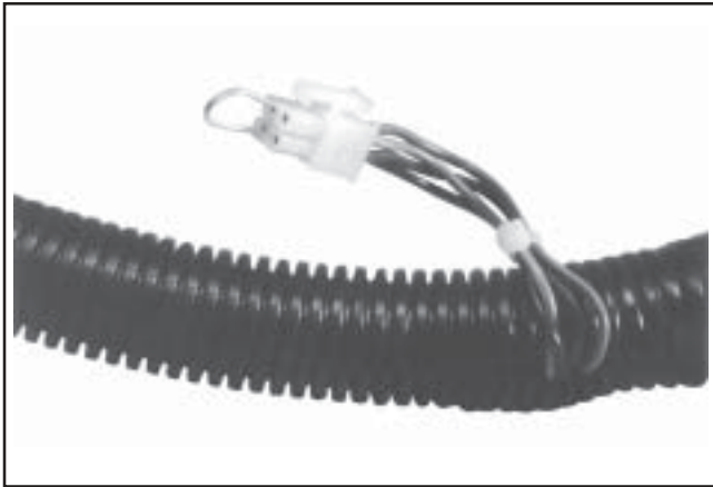
Figure 5B-8. Service Connector Plug, Metal-Cased ECU Harness.
