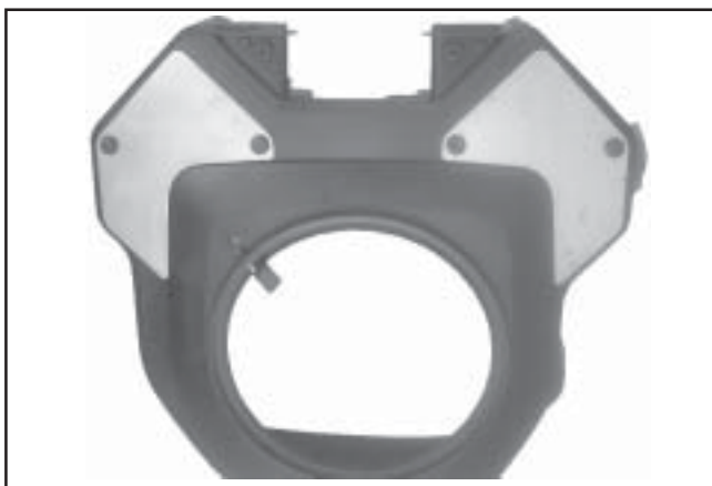
Figure 4-15. Cleanout Kit Installed on Blower Housing.
