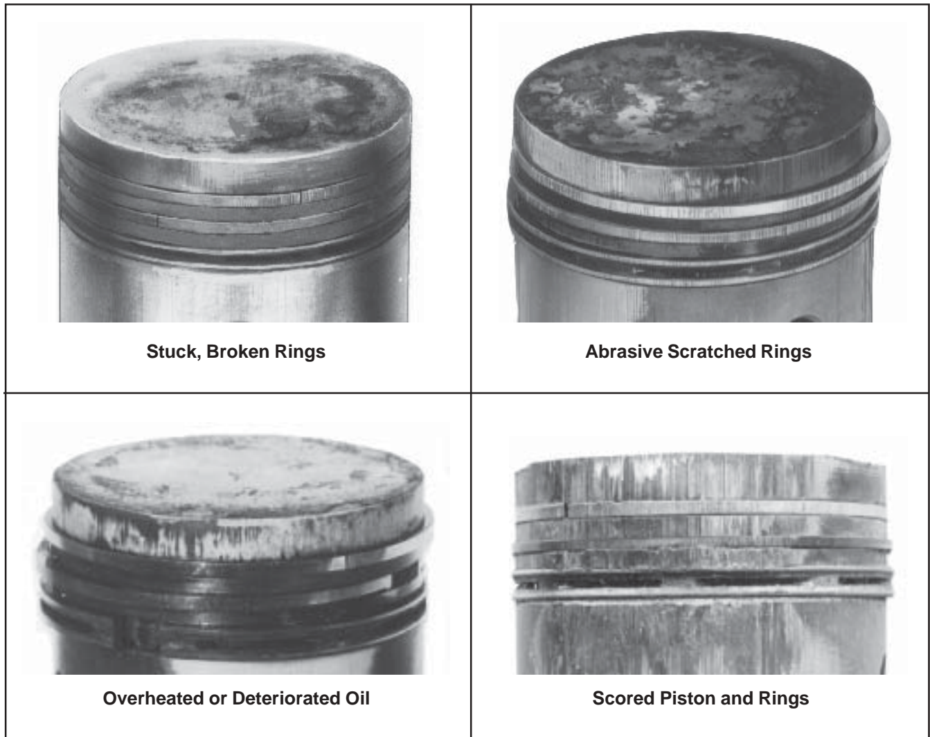
Figure 10-8. Common Types of Piston Damage.
