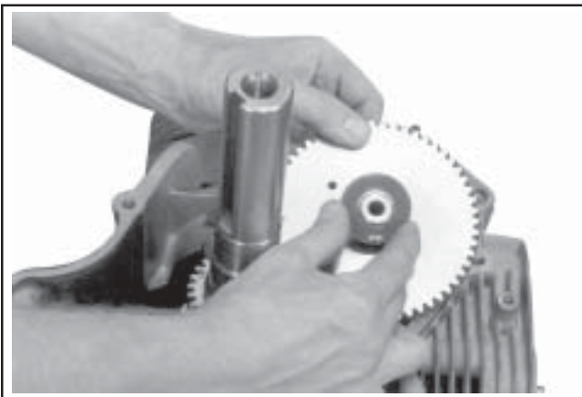
Figure 11-15. Change Shim to Obtain Correct End Play.
