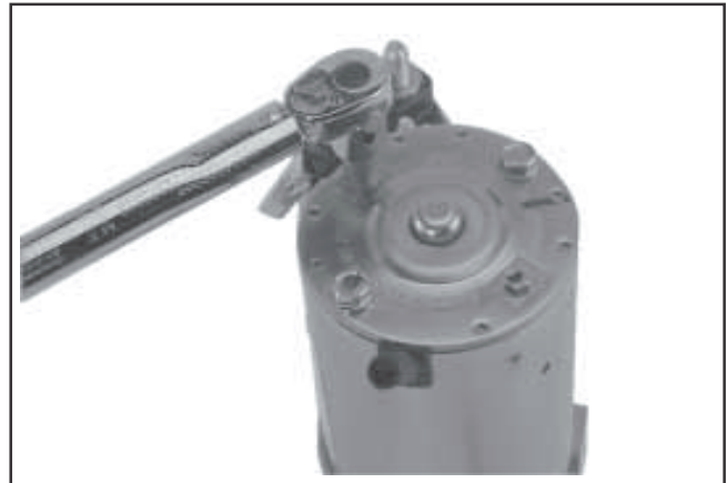
Figure 7-44. Torquing Brush Holder Screws.
