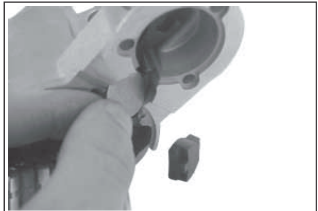
Figure 7-23. Removing Backing Plate and Pivot Bushing.
