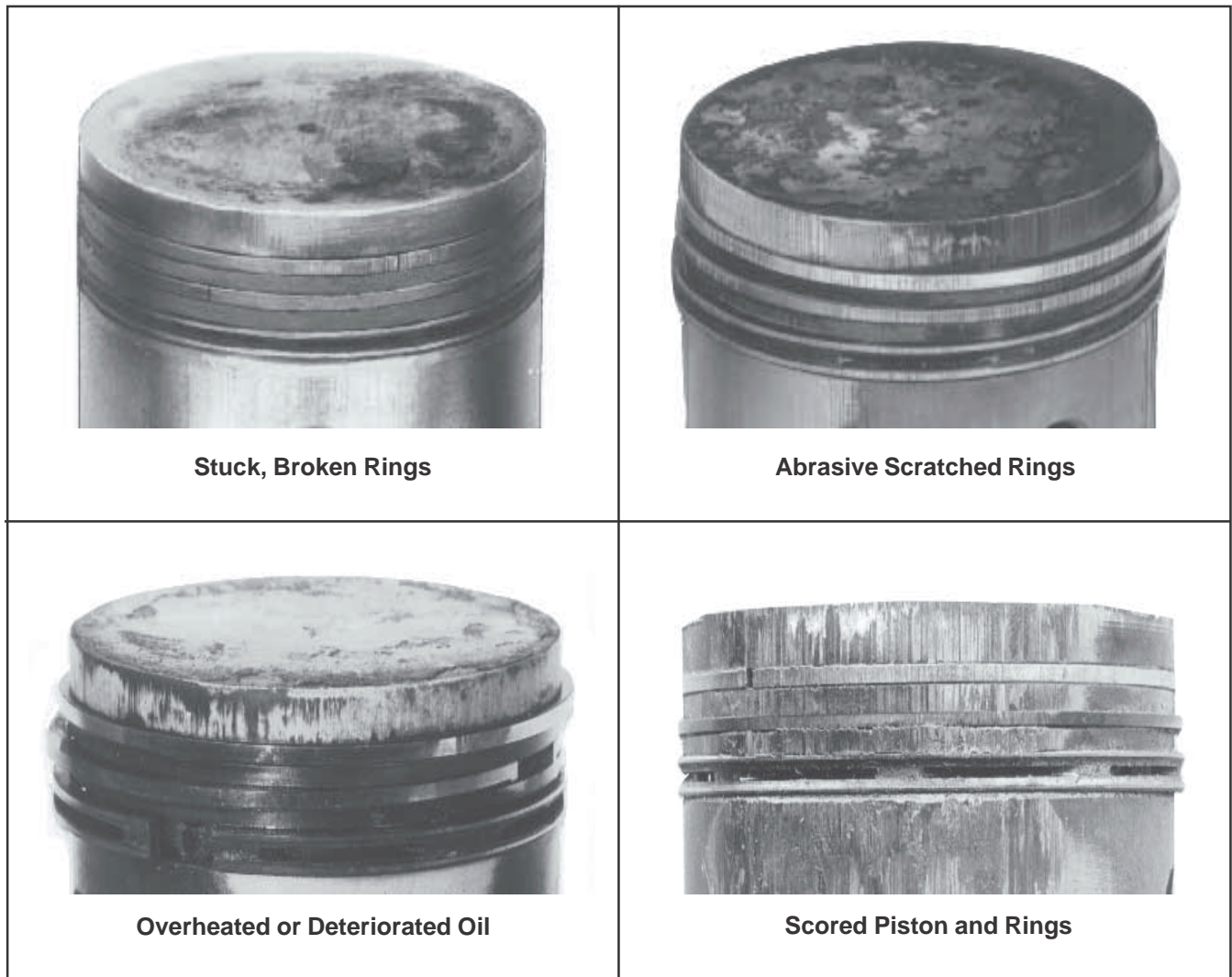
Figure 9-8. Common Types of Piston and Ring Damage.
