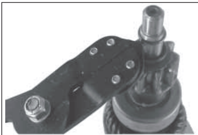
Figure 7-26. Removing Retaining Ring.
