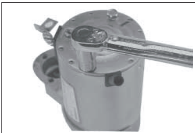
Figure 7-43. Torquing Thru Bolts.
