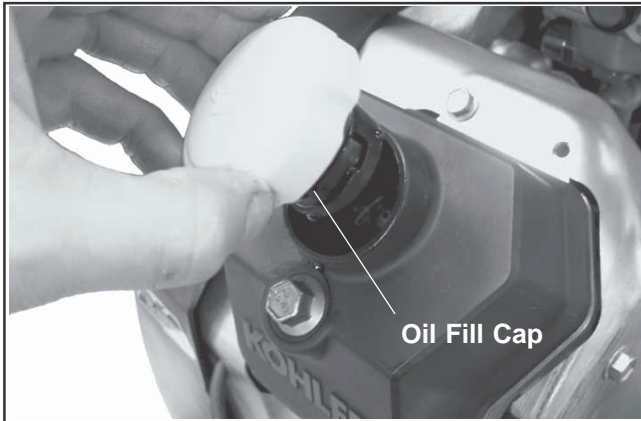
Figure 6-6. Removing Oil Fill Cap.
