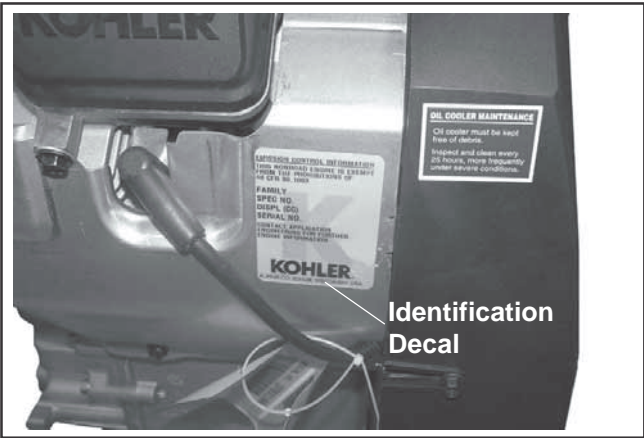
Figure 1-1. Engine Identification Decal Location.
