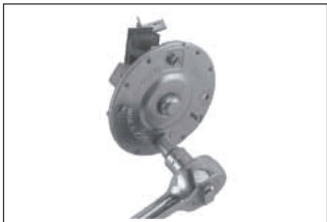
Figure 7-31. Removing Brush Holder.
