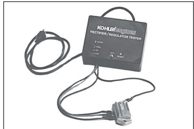
Figure 7-14. Tester Connected to 15 Amp Rectifier-Regulator.
