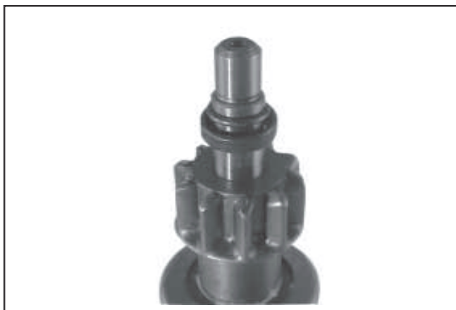
Figure 7-25. Retaining Ring Detail.
