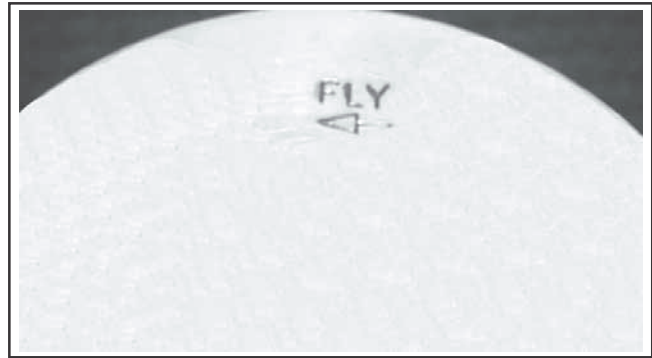
Figure 10-18. FLY Mark on Piston.
