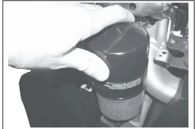
Figure 10-112. Installing Oil Filter.
