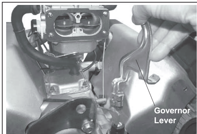
Figure 8-13. Removing Governor Lever.
