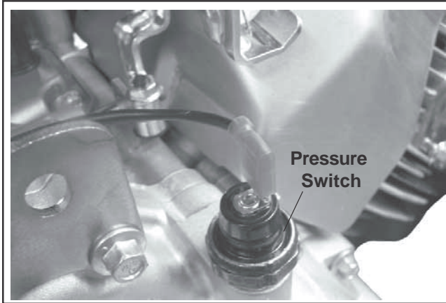
Figure 8-15. Oil Sentry™ Switch Location in Closure Plate.
