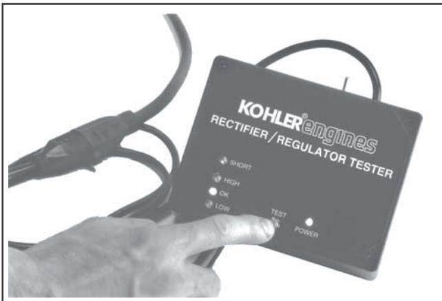
Figure 7-13. Pressing Test Button.
