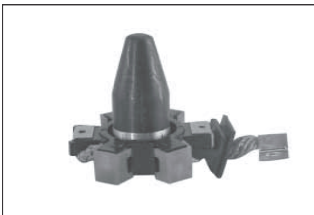
Figure 7-41. Brush Installation Tool with Extension.
