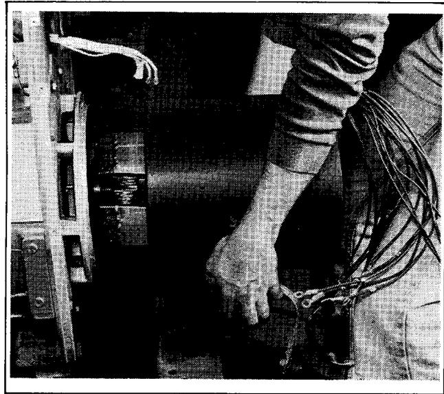
Figure 4-13. Stator Removal
