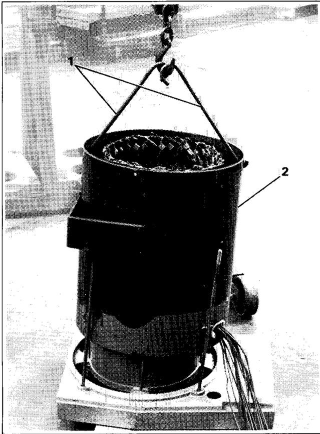
1. Lifting Hooks    2. Stator
