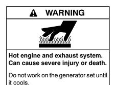
Servicing the exhaust system. Hot parts can cause severe injury or death. Do not touch hot engine parts. The engine and exhaust system components become extremely hot during operation.
