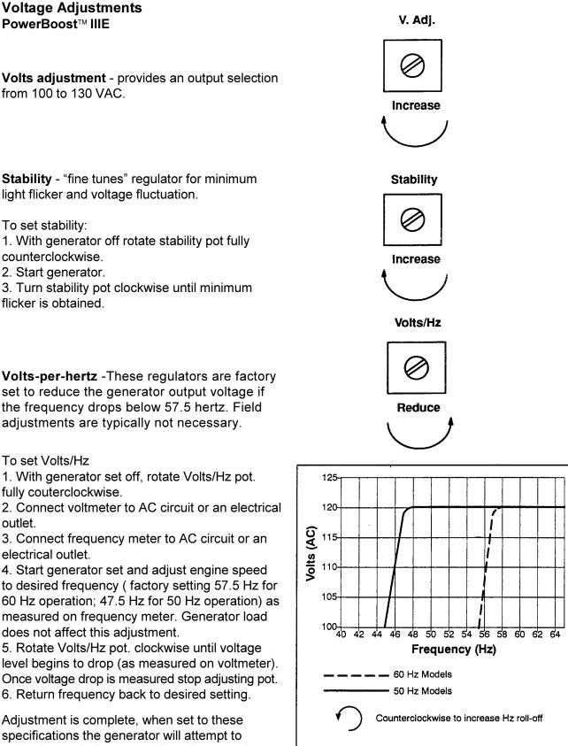
maintain nominal output until engine speed drops to the adjusted cutout point.
