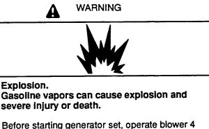
Before starting generator set, operate blower 4 minutes and check engine compartment for gasoline vapors.
