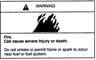
A flash fire can cause severe injury or death. Do not Smoke or permit flame or spark to occur near carburetor, fuel line, fuel filter, fuel pump, or other potential sources of spilled fuel or fuel vapors. When removing fuel line or carburetor, use a proper container to catch all fuel.
