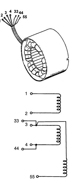
Note: Use same procedure on three phase 12 lead generators.
