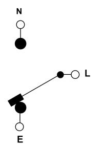
An electric solenoid operates the linkage to flip the moveable contact between the power sources. A complete transfer occurs within 50 milliseconds.
