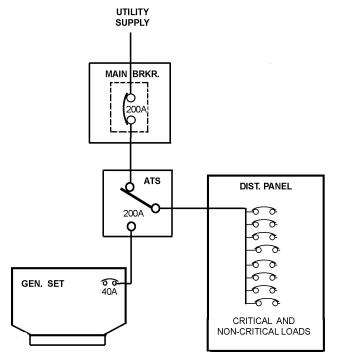
The load applied to the generator can be reduced if required by manually opening distribution breakers.
