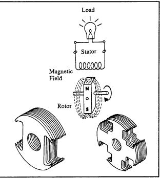
The number of poles and the rotational speed will determine the frequency of the generated output potential.
