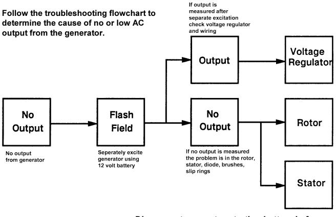
Disconnect generator starting battery before testing any parts of the alternator assembly!!!!
