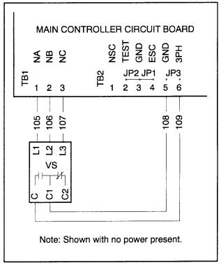
Cut JP3 when using three-phase voltage sensing module.
