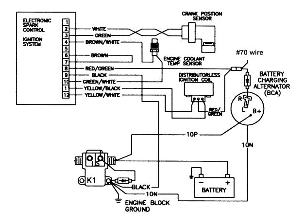
The #70 wire is required to the ESC Module (input terminal 8) and also to the DIS coil. The #70 wire is electrically hot (battery voltage) when the generator is in the crank or run mode. A ground is also required to terminal 9 of the ESC module.
