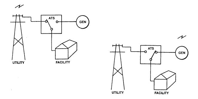
The system concept features a utility (primary) source, generator (backup) source, and an automatic transfer switch connected to a building load.
