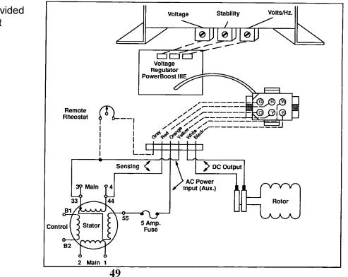
A 5-amp fuse (F2) is provided to protect the power input circuit. (55)
