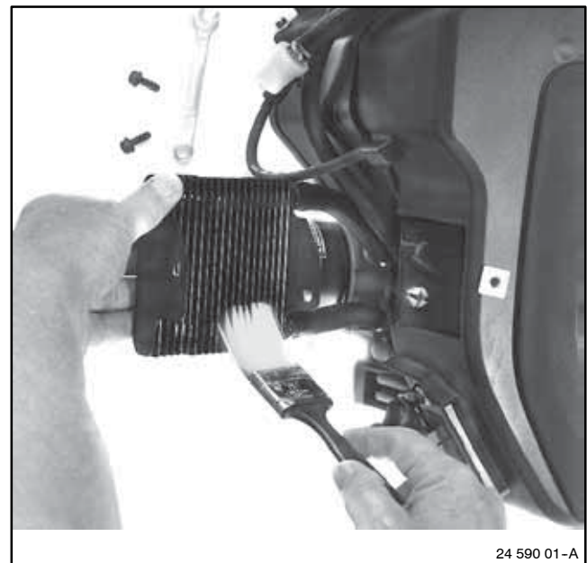
Figure 2-6 Cleaning the Oil Cooler
