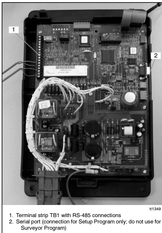
Figure 1-3 ATS Controller (cover removed)
