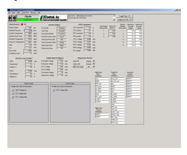
The System Fault screen is used to view and clear DTC's that have been set.
