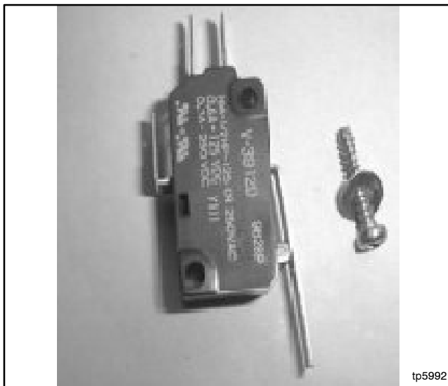
Figure 6-11 Microswitch and Mounting Screw
