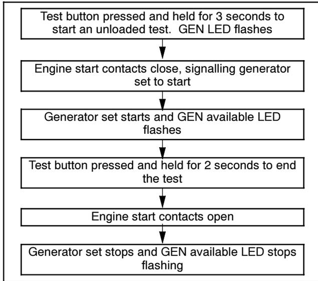
**Figure 2-9** Unloaded Test Sequence
