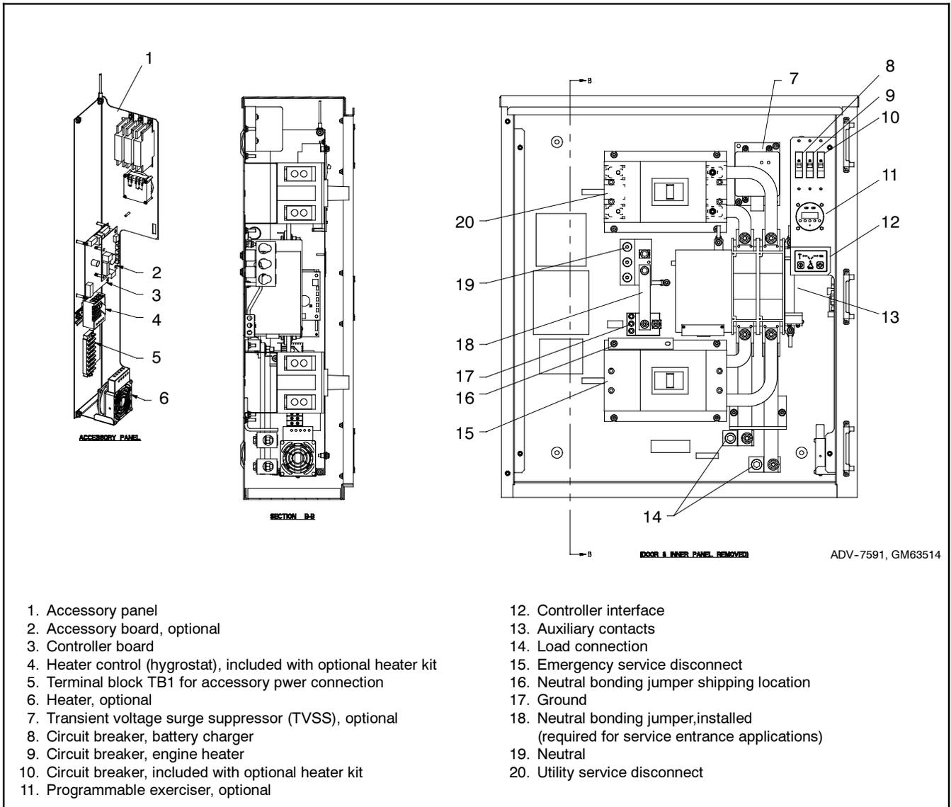
**Figure 1-10** 400 Amp Service Entrance Model Components
