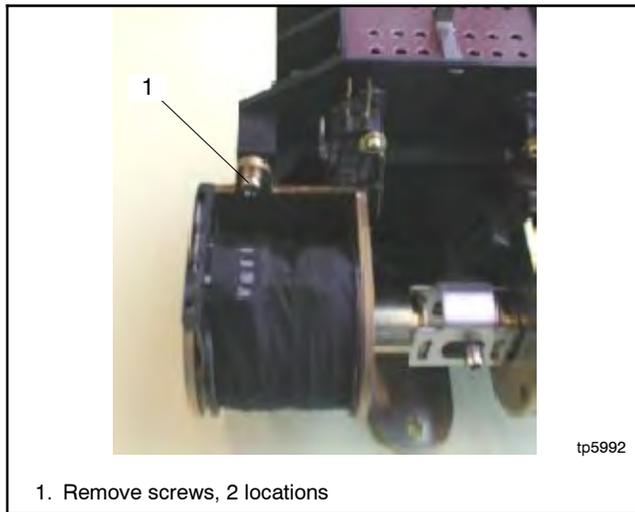
**Figure 7-6** Solenoid Assembly
