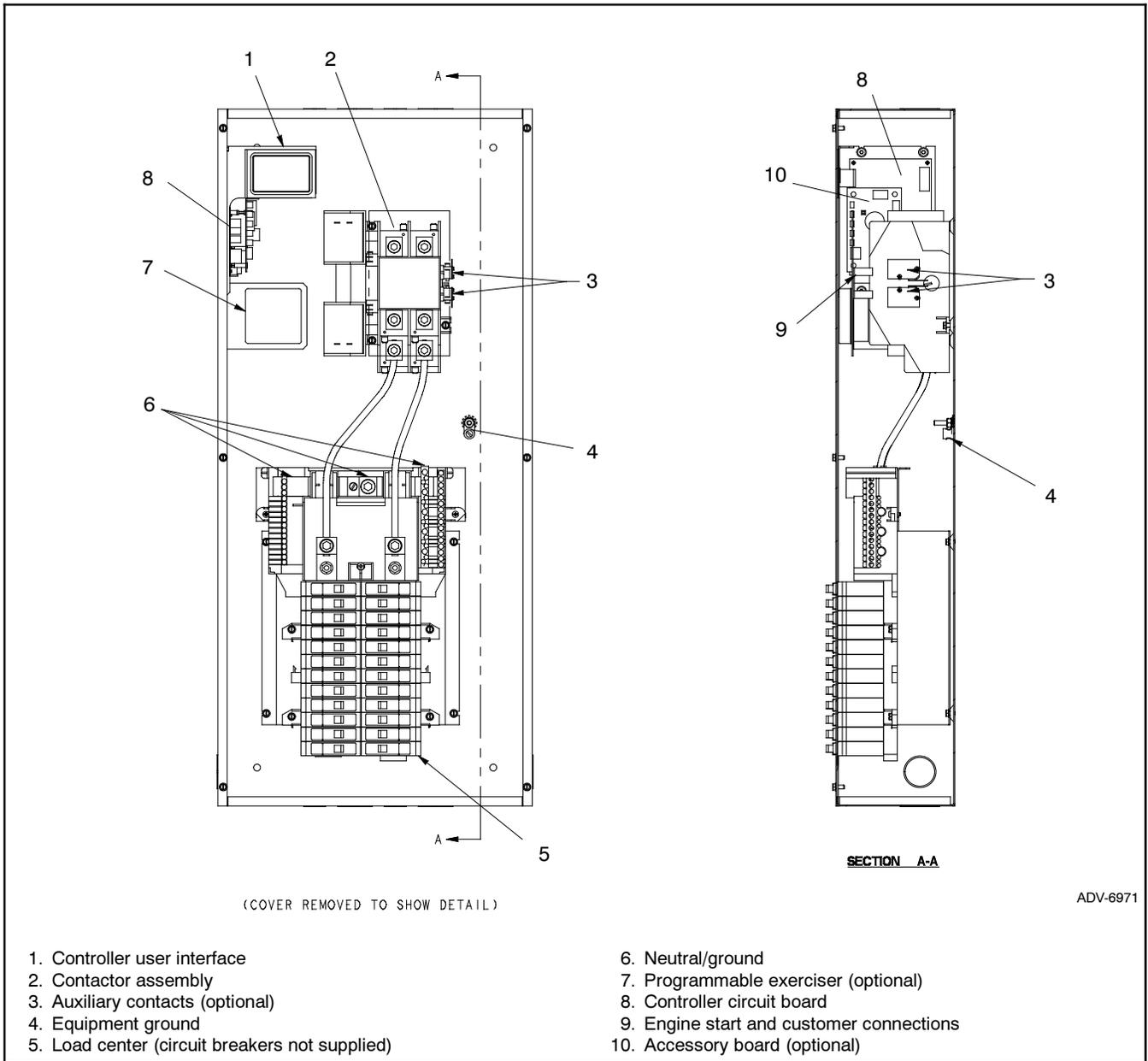
**Figure 1-7** 200 Amp Model with Load Center Components
