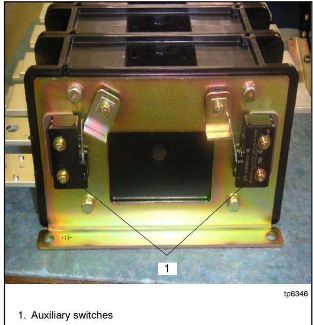
**Figure 7-32** Auxiliary switch Location
