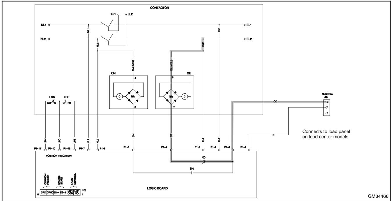
**Figure 5-17** Normal to Emergency, 100/200 Amps. Transfer Switch in Normal Position, Normal Source Not Available, Emergency Available. After Normal-to-Emergency Time Delay, ATS Transfers to Emergency Position.
