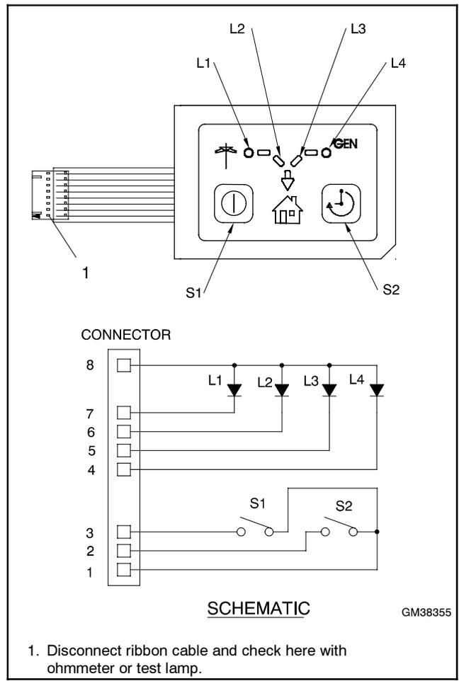
Figure 5-10 Switch/LED Membrane
