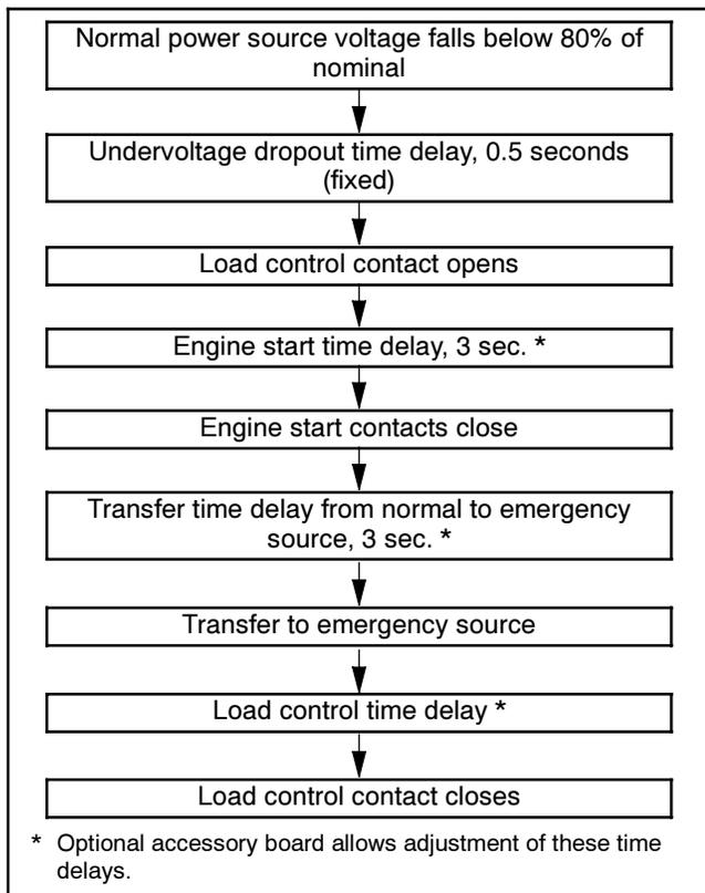
**Figure 2-7** ATS Sequence of Operation, Transfer to Emergency
