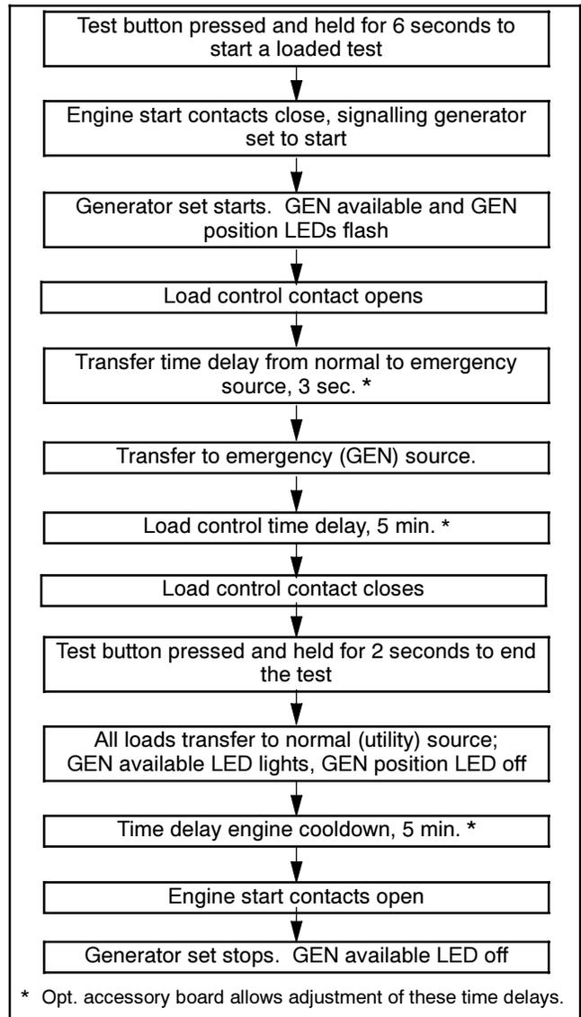
**Figure 2-10** Loaded Test Sequence
