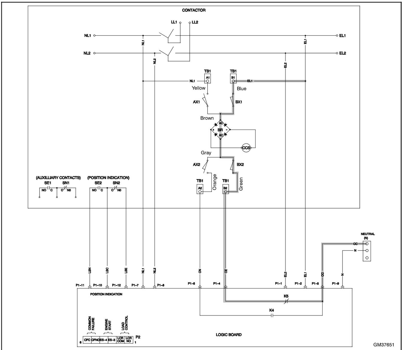
**Figure 5-19** Normal to Emergency, 400 Amp Models. Transfer Switch in the Normal Position, Normal Fails, Emergency Available. After Normal-to-Emergency Time Delay, ATS Transfers to the Emergency Position
