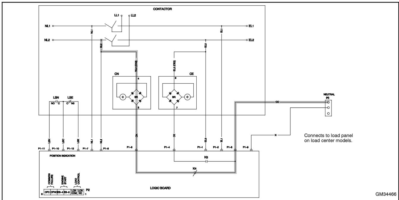
**Figure 5-18** Emergency to Normal, 100/200 Amp Models. Transfer Switch in Emergency Position, Emergency Present, Normal Returns. After Emergency-to-Normal Time Delay, the ATS Transfers to Normal Position
