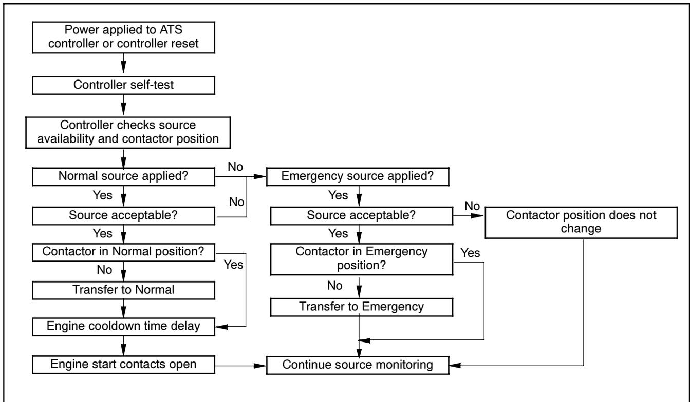
Figure 2-6 Powerup/Reset Sequence
