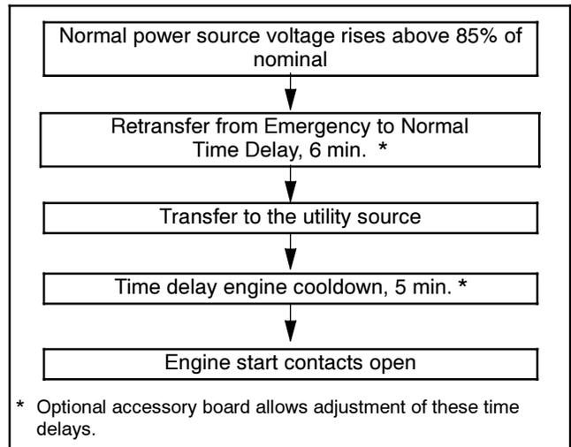
**Figure 2-8** ATS Sequence of Operation, Retransfer to Normal
