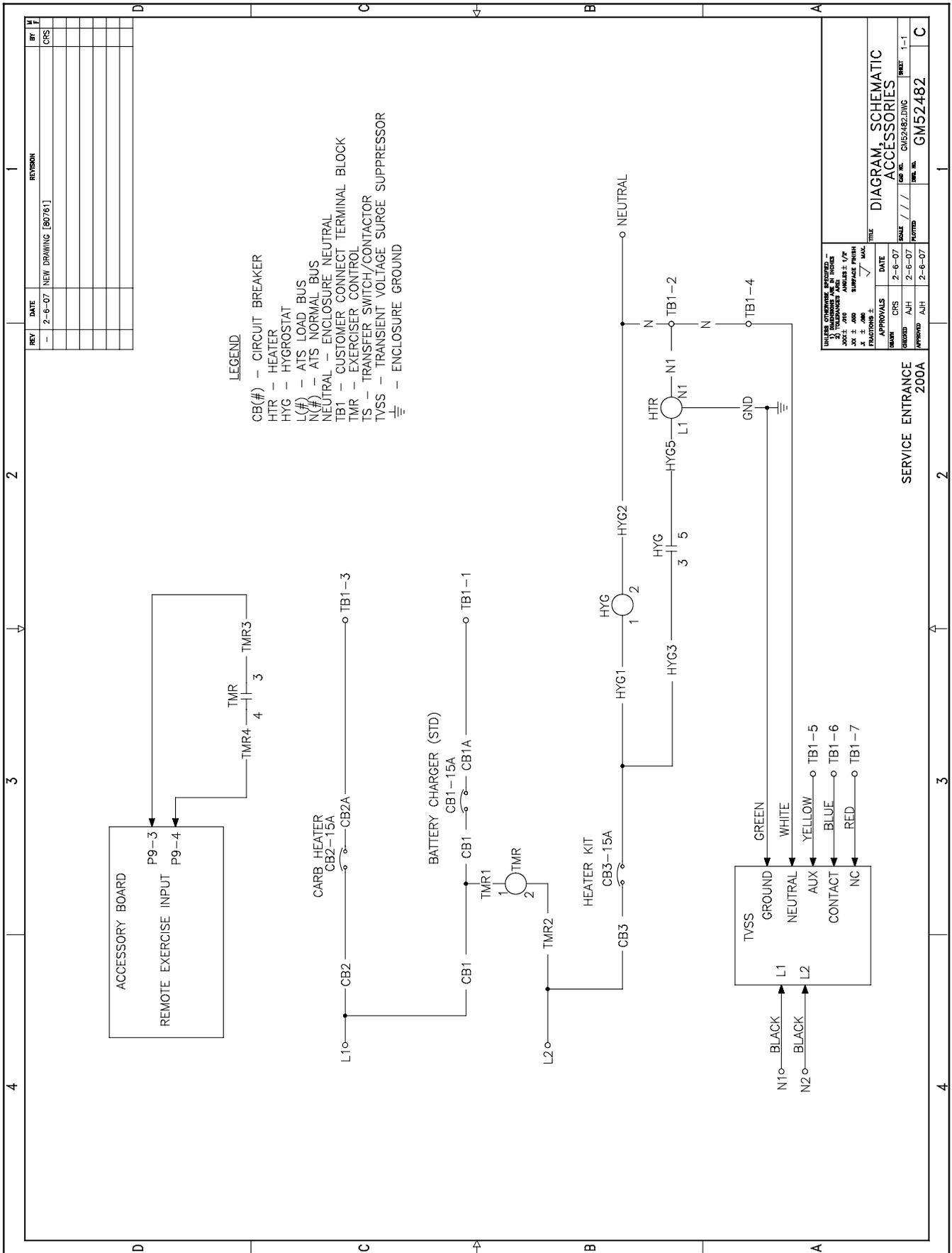
Figure 6-11 Schematic Diagram, 200 Amp Service Entrance Switch Accessories, GM52482
