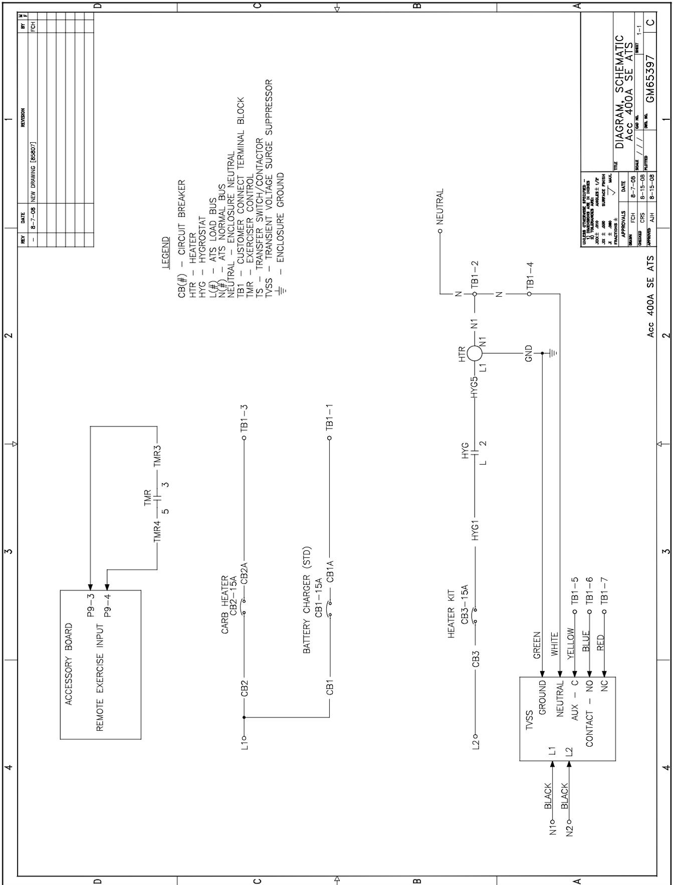
Figure 6-16 Schematic Diagram, 400 Amp Service Entrance Switch Accessories, GM65397
