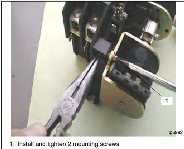
1. Install and tighten 2 mounting screws
