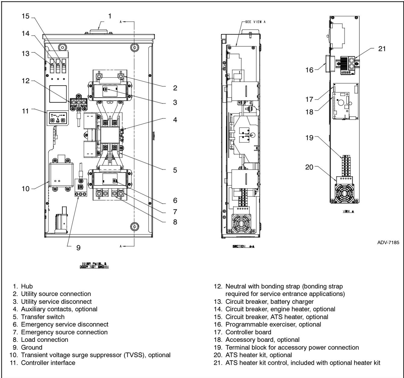
**Figure 1-9** 200 Amp Service Entrance Model Components
