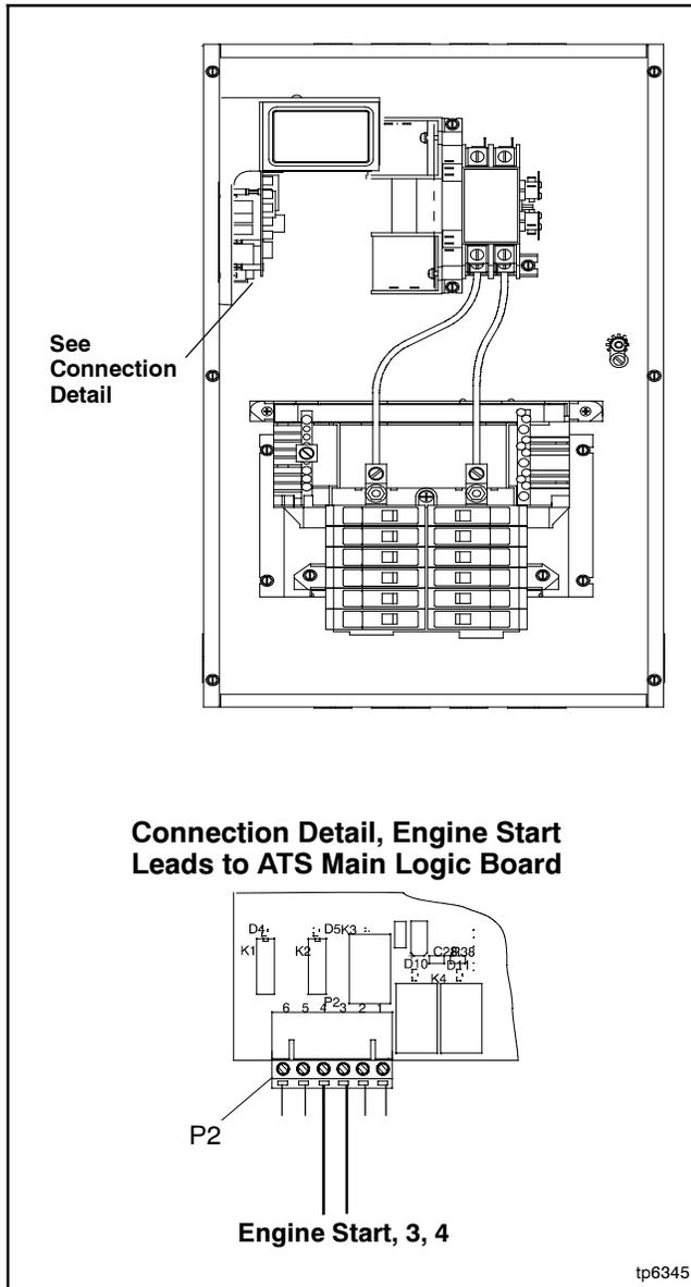
**Figure 5-11** Engine Start Connection
