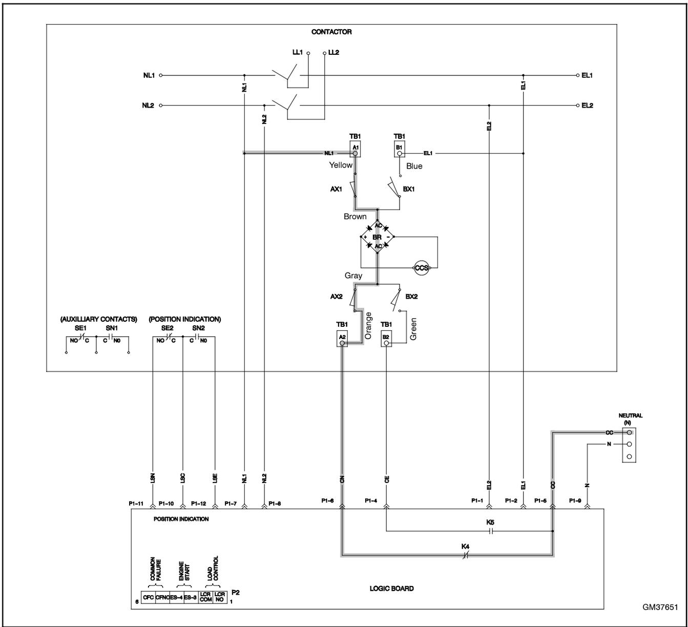
**Figure 5-20** Emergency to Normal, 400 Amp Models. Transfer Switch in the Emergency Position, Emergency Present, Normal Returns, ATS Transfers to the Normal Position
