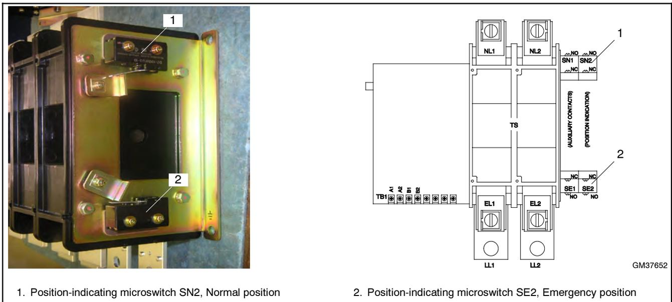
**Figure 5-14** Position-Indicating Microswitches, 400-Amp Models
