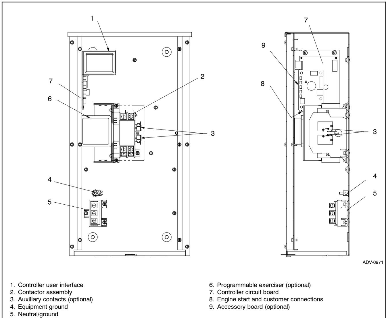
**Figure 1-6** 100 Amp Model without Load Center Components
