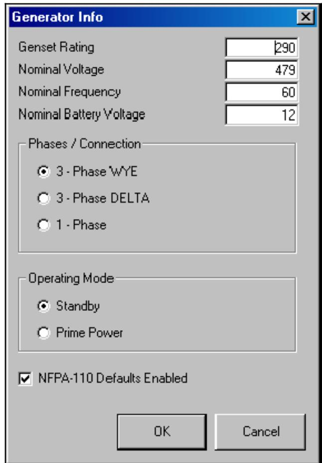
Figure 3-15 Generator Info Setup Window
