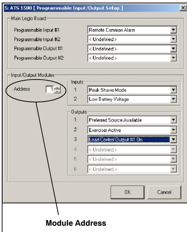
Figure 7-26 Programmable Input/Output Setup
