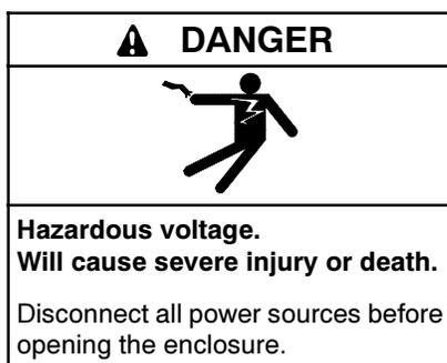
**Opening the power monitor enclosure. Hazardous voltage can cause severe injury or death.** A transfer switch or generator set connected to the power monitor could automatically energize the power monitor or accessories. Disconnect all power sources before opening the enclosure. Move the generator set master switch on the controller to the OFF position and disconnect the battery negative (-) lead before proceeding.
