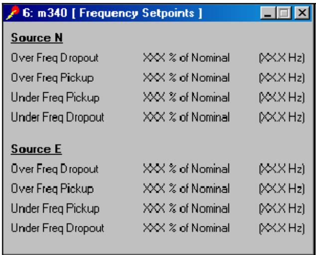
Figure 9-3 Frequency Setpoints Window
