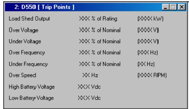
Figure 3-24 Trip Point Display Window
