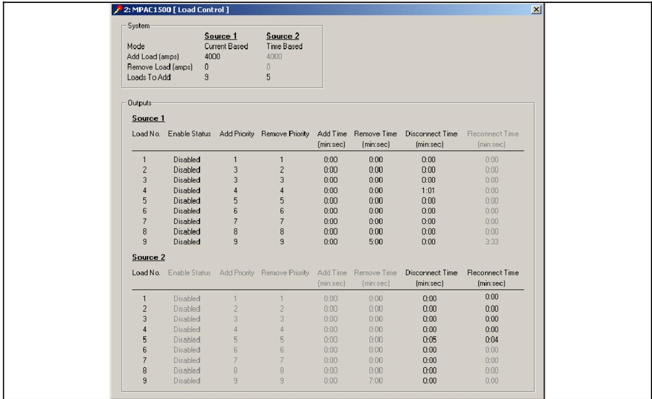
**Figure 7-15** Load Control Display, Monitor III Version 3.0.0 or Higher (showing current-based load control for Source 1 and time-based load control for Source 2.)
