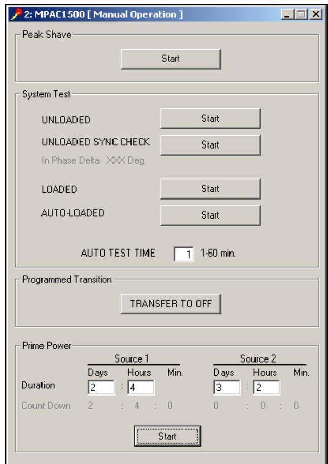
**Figure 7-23** Manual Operation, version 3.0.0 or higher
