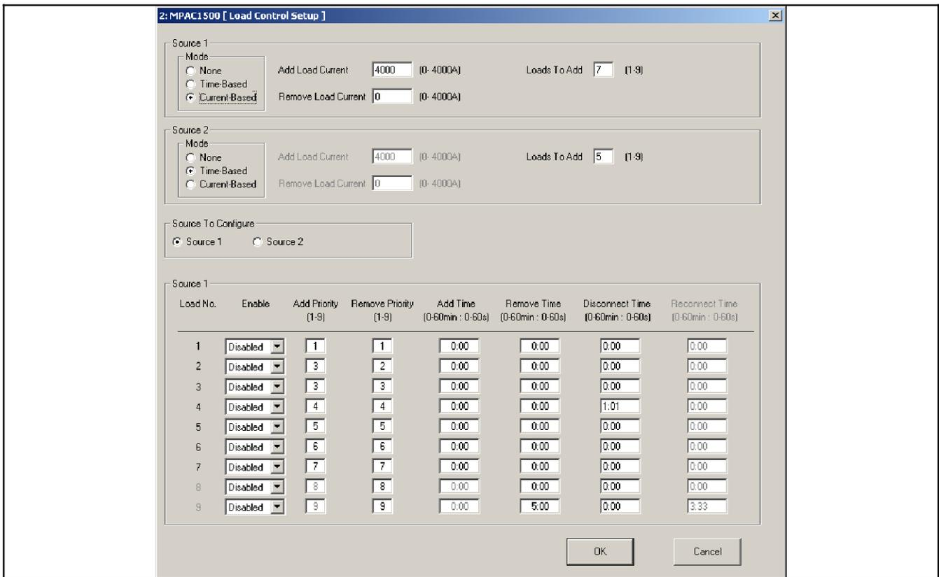
**Figure 7-16** Load Control Setup, Monitor III Version 3.0.0 or Higher (showing current-based load control for Source 1)
