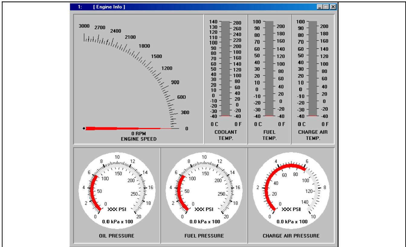
Figure 5-8 Engine Info Window (engines equipped with ECMs)
