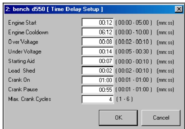
Figure 3-23 Time Delay Setup Window
