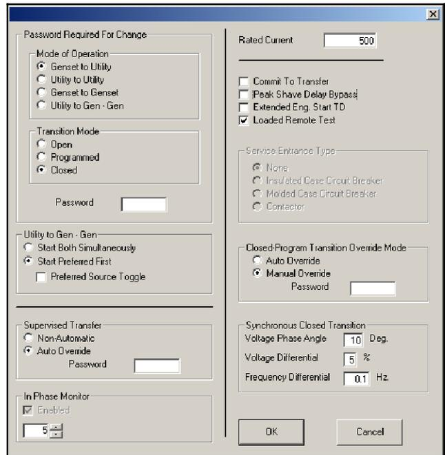
Figure 7-41 System Summary Setup Window, Monitor III versions 3.0.0 or higher
