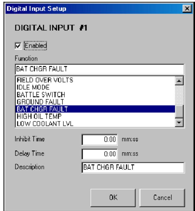
**Figure 3-9** Digital Input Setup Window for a Single Digital Input
