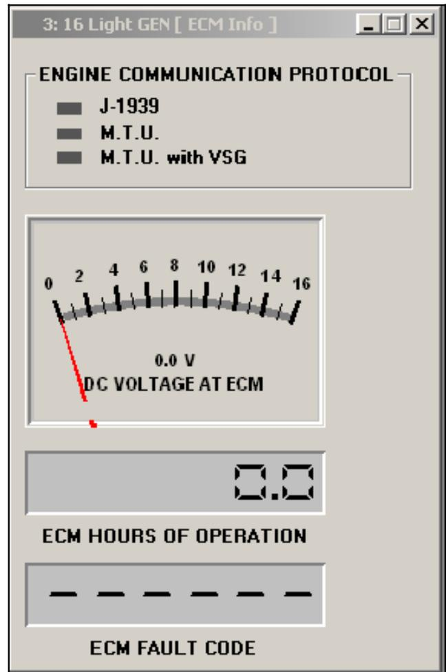
**Figure 5-5** ECM Info Display Window (for engines equipped with ECMs)
