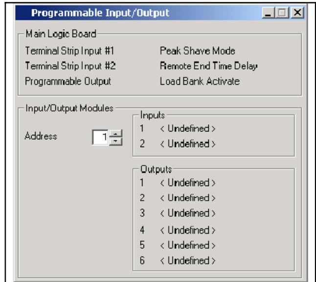
**Figure 8-19** Programmable Input/Output Display
