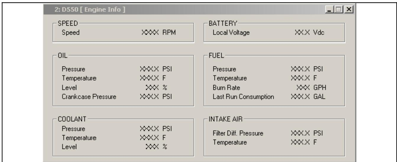
Figure 3-12 Engine Info Display Window
