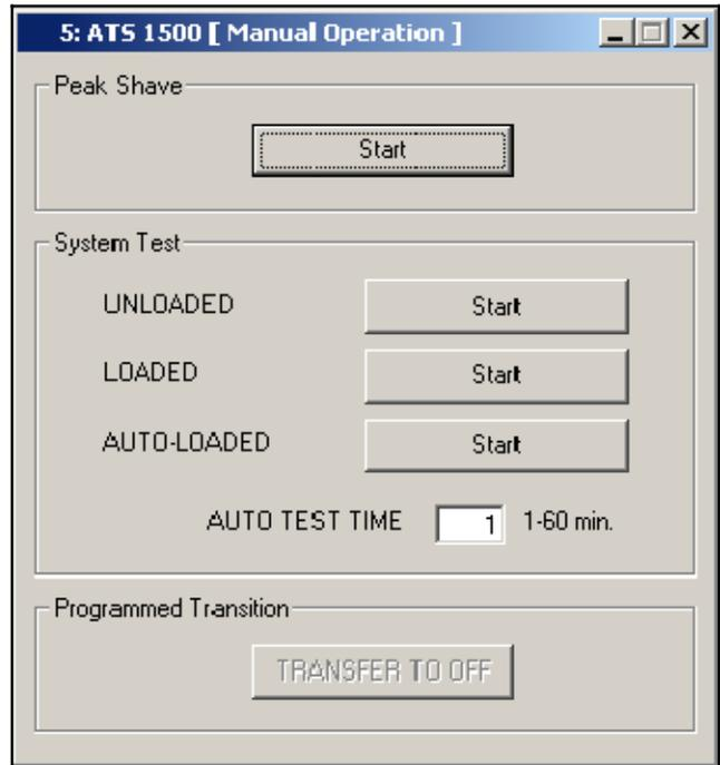
**Figure 7-22** Manual Operation, prior to version 3.0.0
