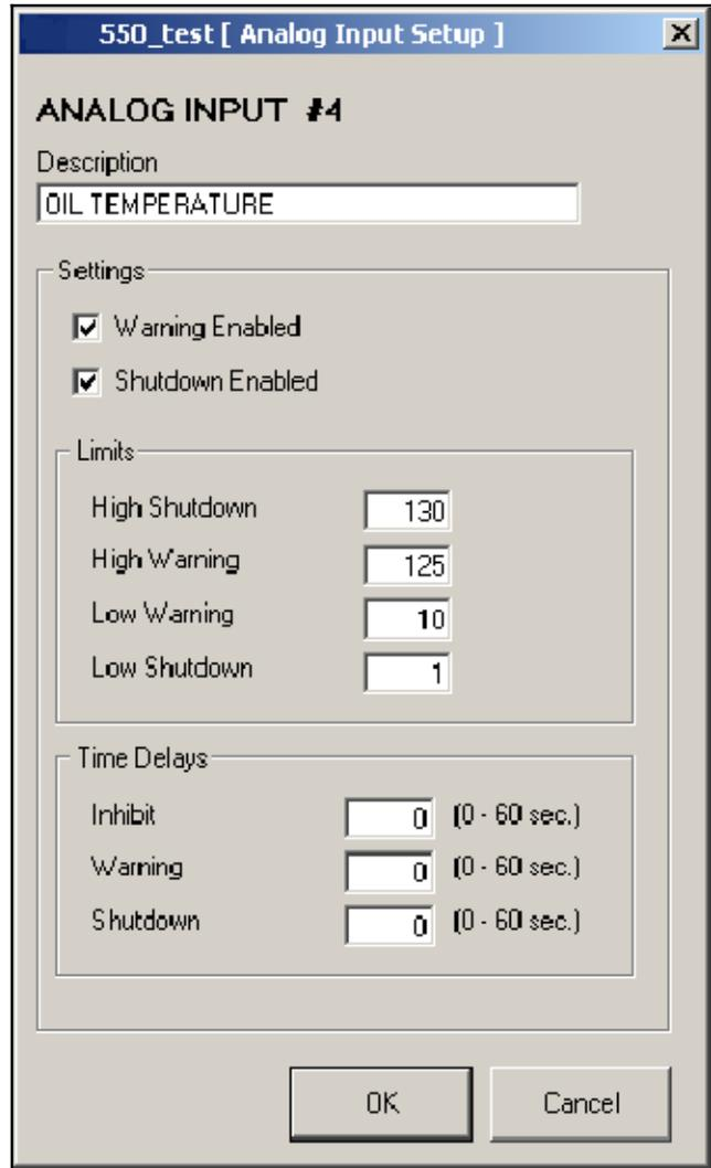
Figure 3-3 Analog Input Setup Window for a Single Analog Input (example settings shown)
