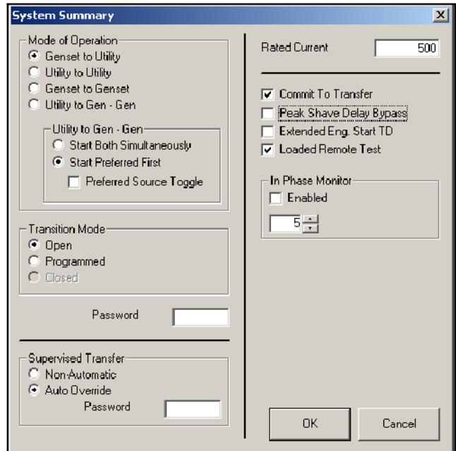
Figure 7-40 System Summary Setup Window, Monitor III prior to version 3.0.0
