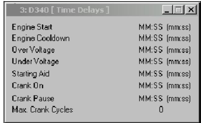
Figure 6-13 Time Delay Window
