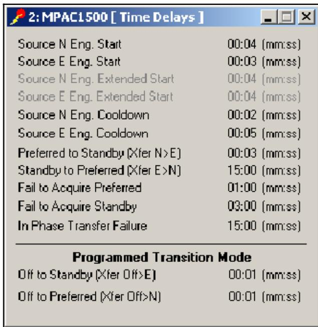
Figure 7-42 Time Delays Display
