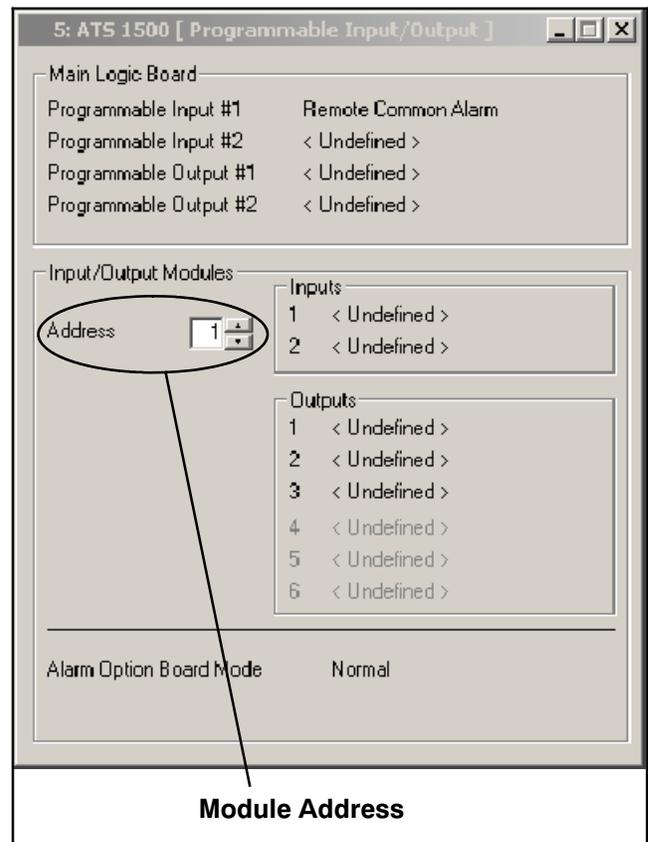
**Figure 7-25** Programmable Input/Output Display
