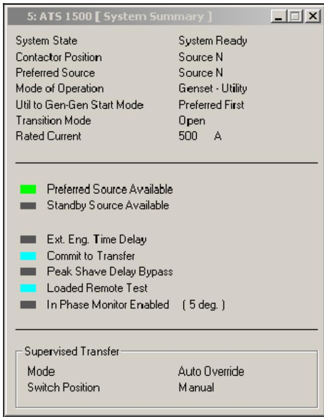
**Figure 7-38** System Summary Display, Monitor III prior to version 3.0.0
