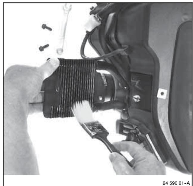
**Figure 3-3** Cleaning Oil Cooler
