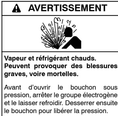
Allow the engine to cool. Release pressure from the cooling system before removing the pressure cap. To release pressure, cover the pressure cap with a thick cloth and then slowly turn the cap counterclockwise to the first stop. Remove the cap after pressure has been completely released and the engine has cooled. Check the coolant level at the tank if the generator set has a coolant recovery tank.
