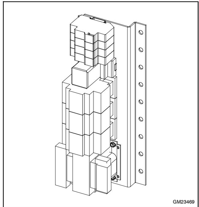
**Figure 8-23** Load Shed Accessory (for identification)
