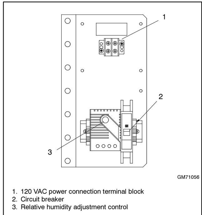
**Figure 8-20** Hygostat Assembly, Typical
