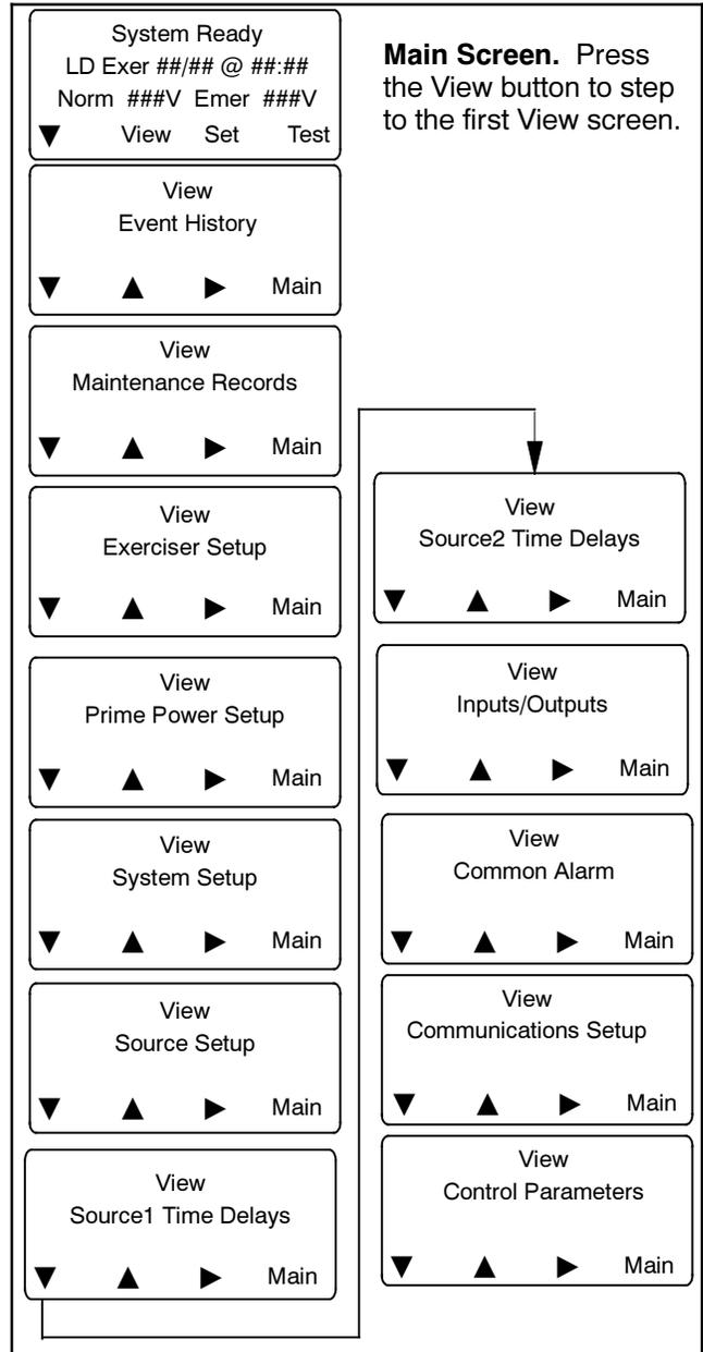
**Main Screen.** Press the View button to step to the first View screen.
