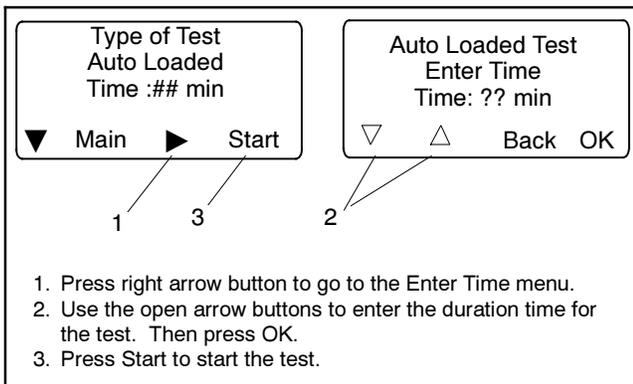
**Figure 3-14** Auto Loaded Test Menus
