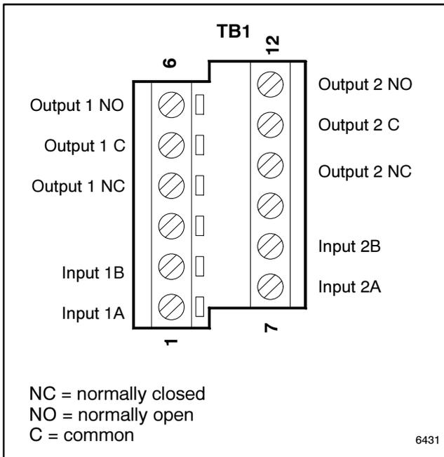
**Figure 1-2** Logic Board Input and Output Connections to TB1
