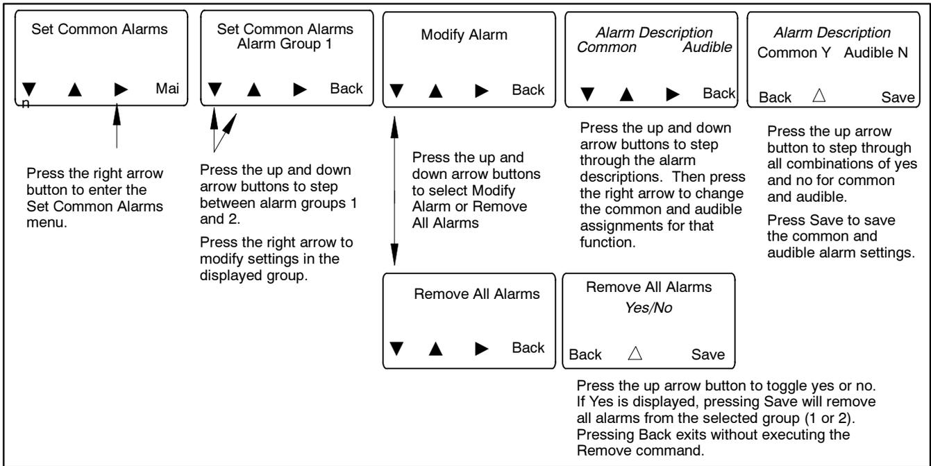
**Figure 3-5** Example: Set Common Alarms
