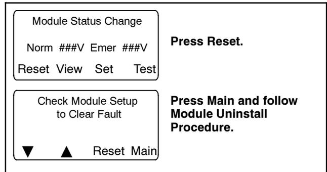
Figure 3-23 Screens after Module Disconnection
