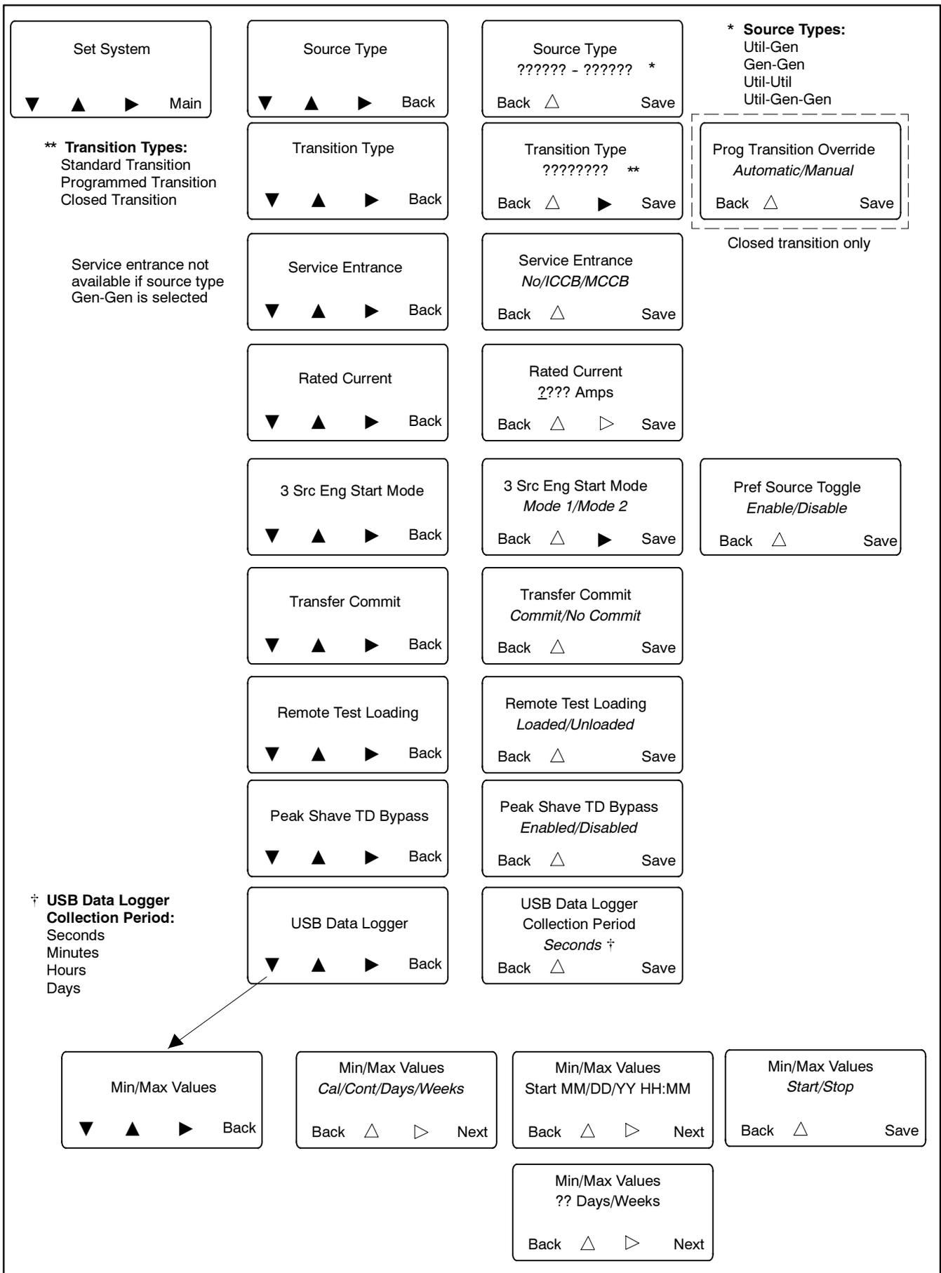
**Figure 5-25** System Setup
