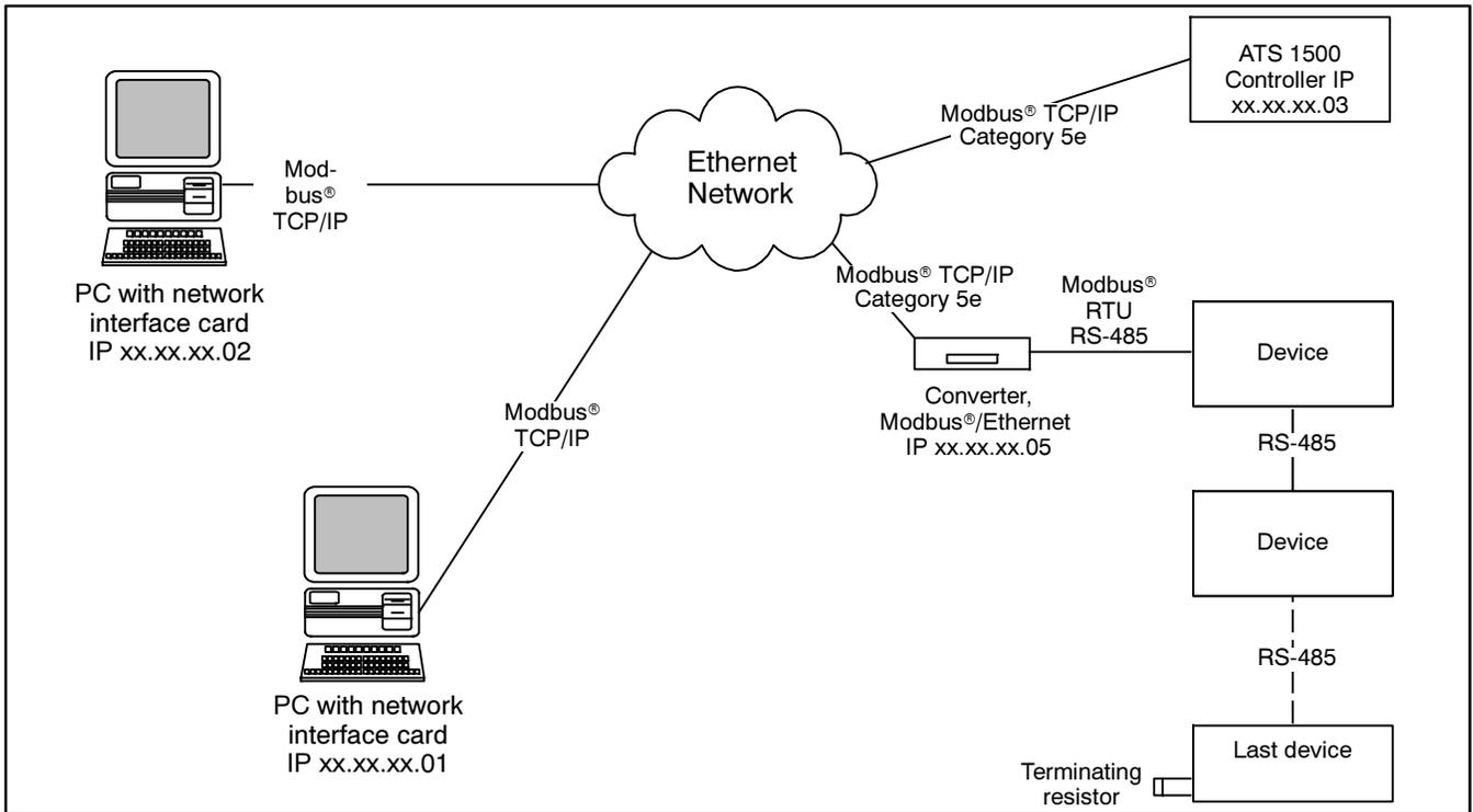
**Figure 6-5** Ethernet Connections to Multiple-Device Network
