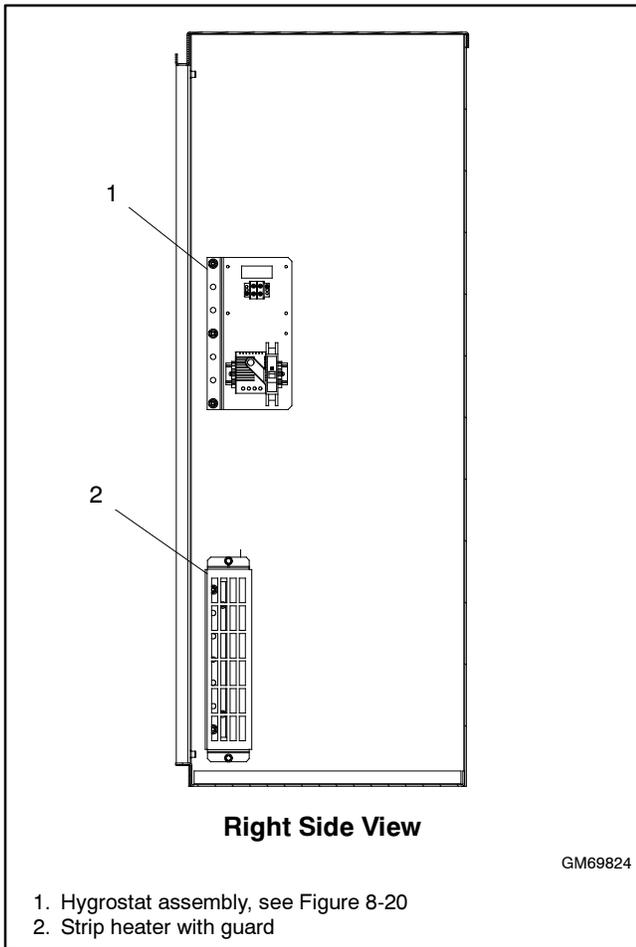
**Figure 8-21** Heater Location, Typical
