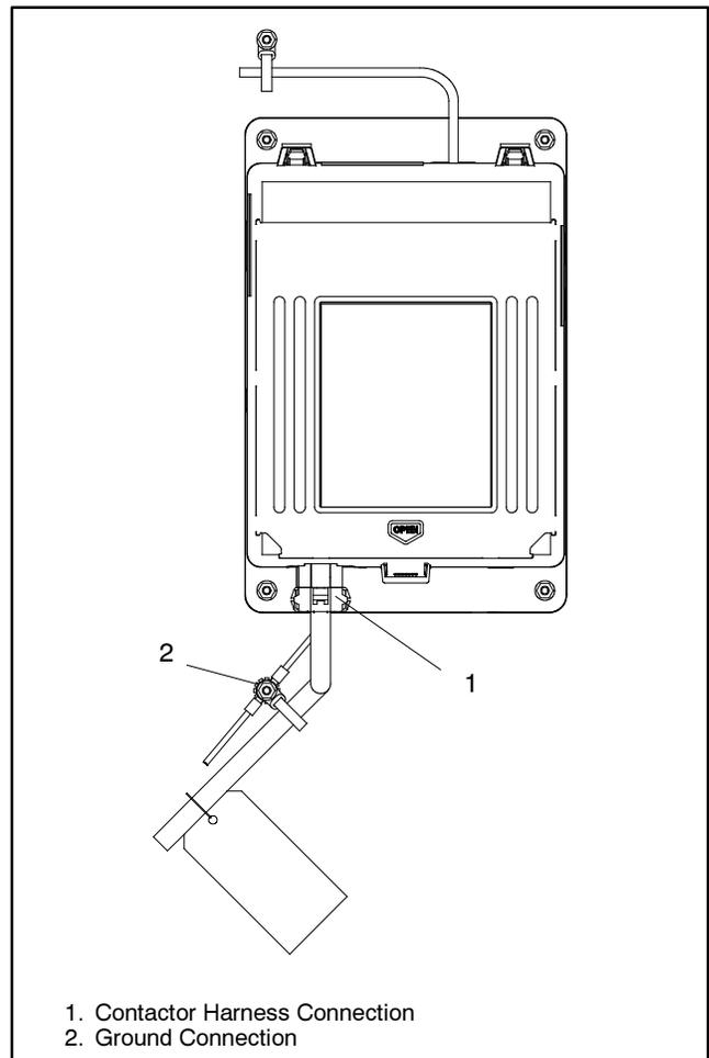
**Figure 1-3** Contactor Harness and Controller Ground Connections
