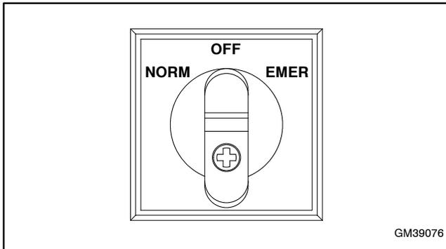
**Figure 8-19** Three-Position Selector Switch
