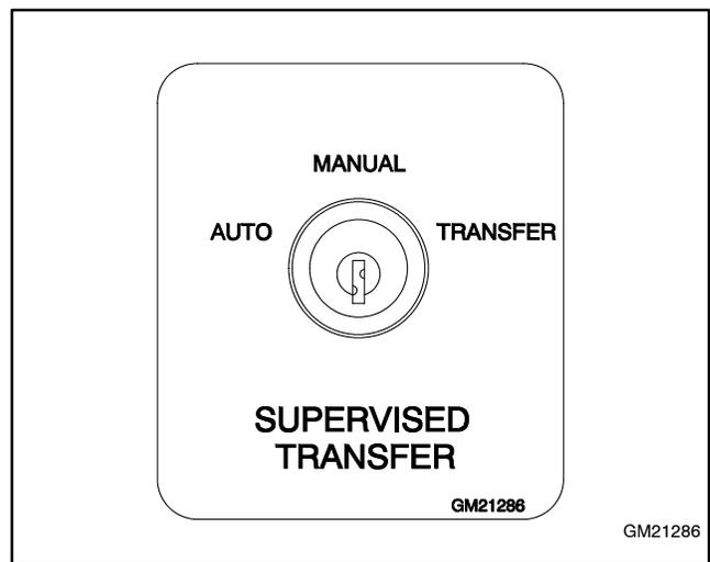
**Figure 8-25** Supervised Transfer Control Switch
