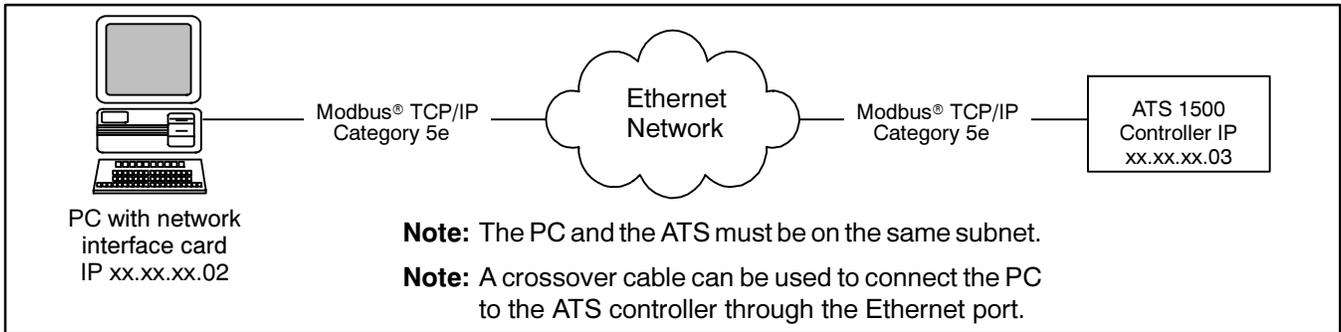
**Figure 6-4** Remote Network (Ethernet) Connection
