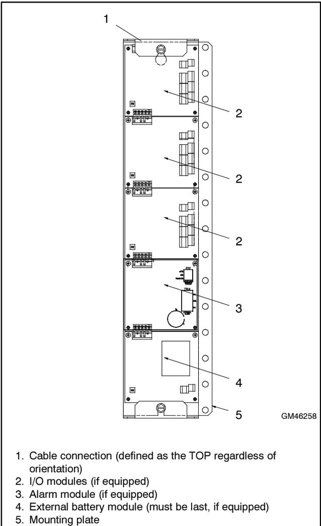
**Figure 8-2** Module Mounting
