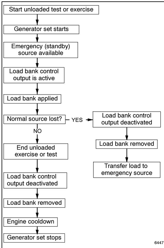
**Figure 5-20** Load Bank Control Sequence
