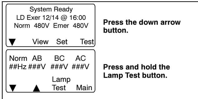
Figure 3-16 Lamp Test
