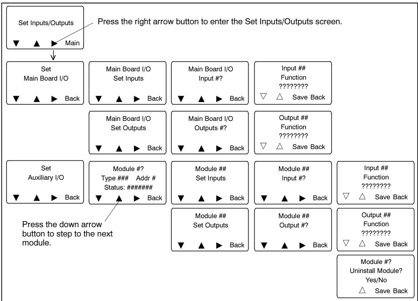
Figure 5-16 Assigning Inputs and Outputs
