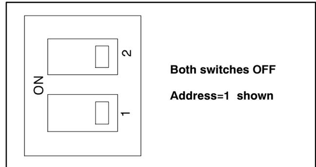
**Figure 8-6** Address DIP Switches
