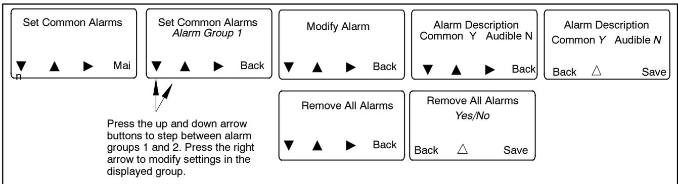
Figure 5-22 Setting Common Alarms
