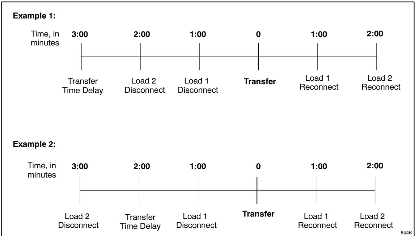
**Figure 5-11** Time-Based Load Control and Transfer Time Delays
