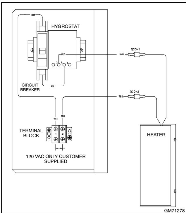
**Figure 8-22** Heater Connections
