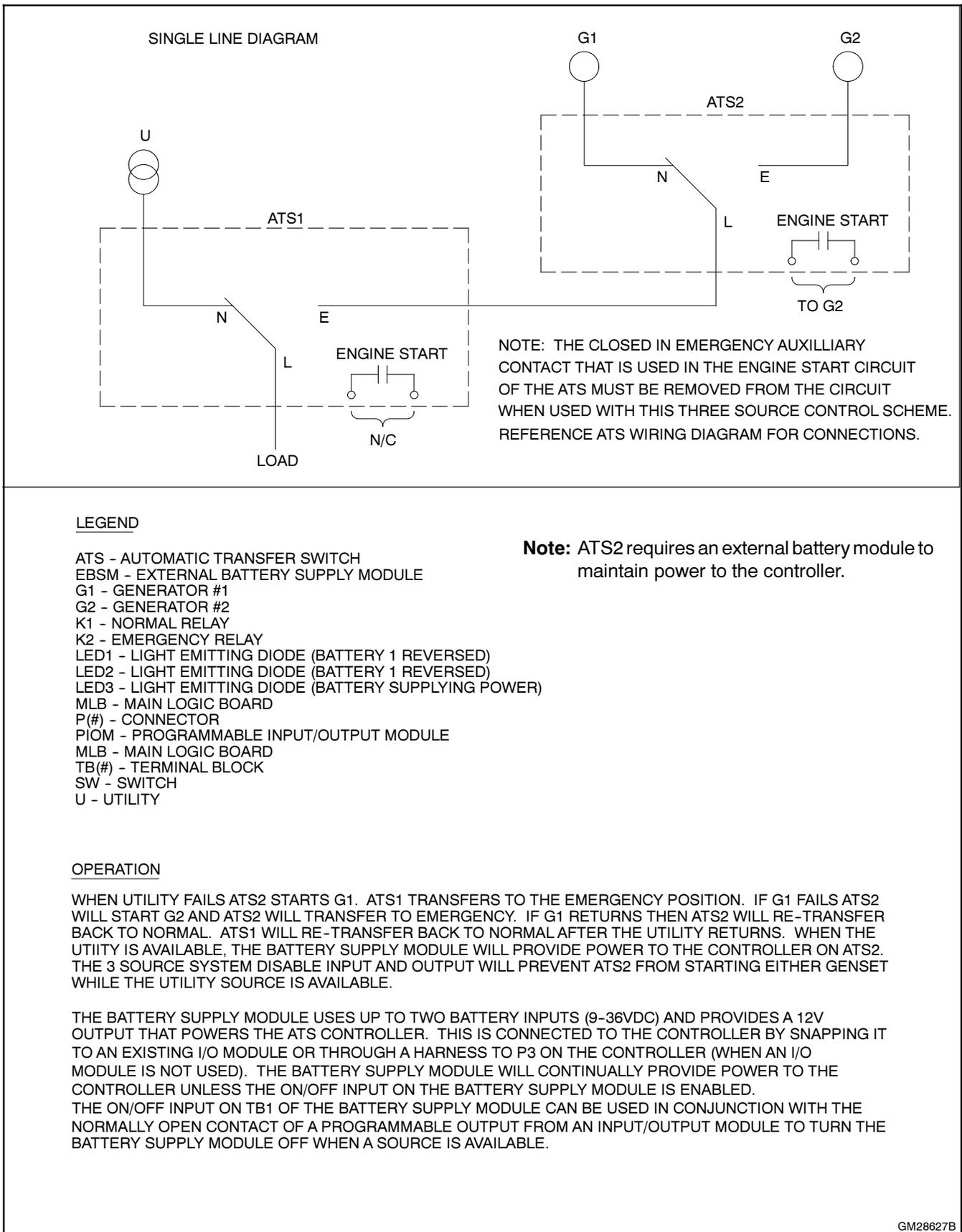
**Figure 5-27** Three-Source System Transfer Switch and Source Connections
