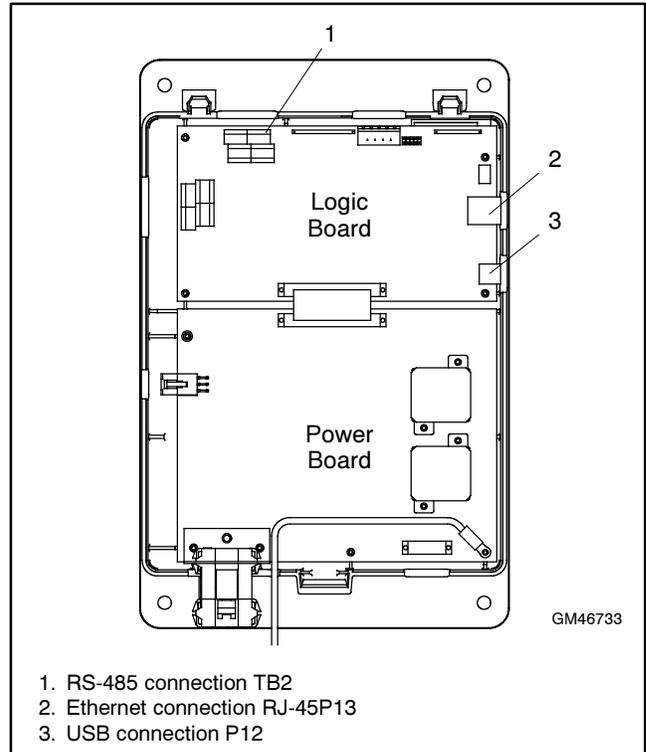
**Figure 6-1** Communication Connections (controller cover removed for illustration only)
