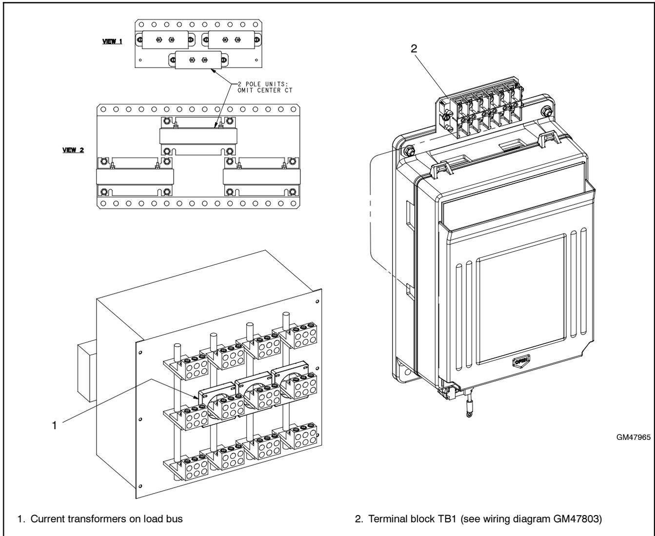
**Figure 8-16** Current Sensing Kit
