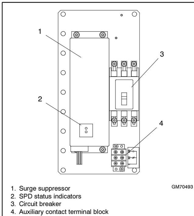
**Figure 8-31** SPD Assembly, Typical
