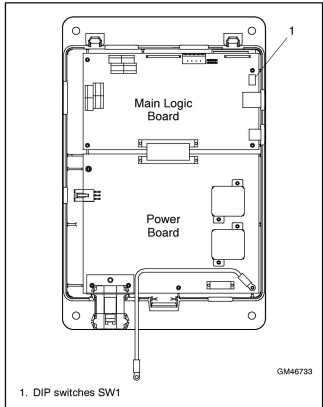
**Figure 5-1** DIP Switch Location (cover removed)
