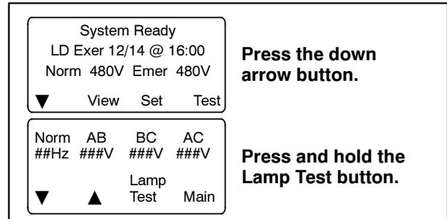
Figure 2-1 Lamp Test
