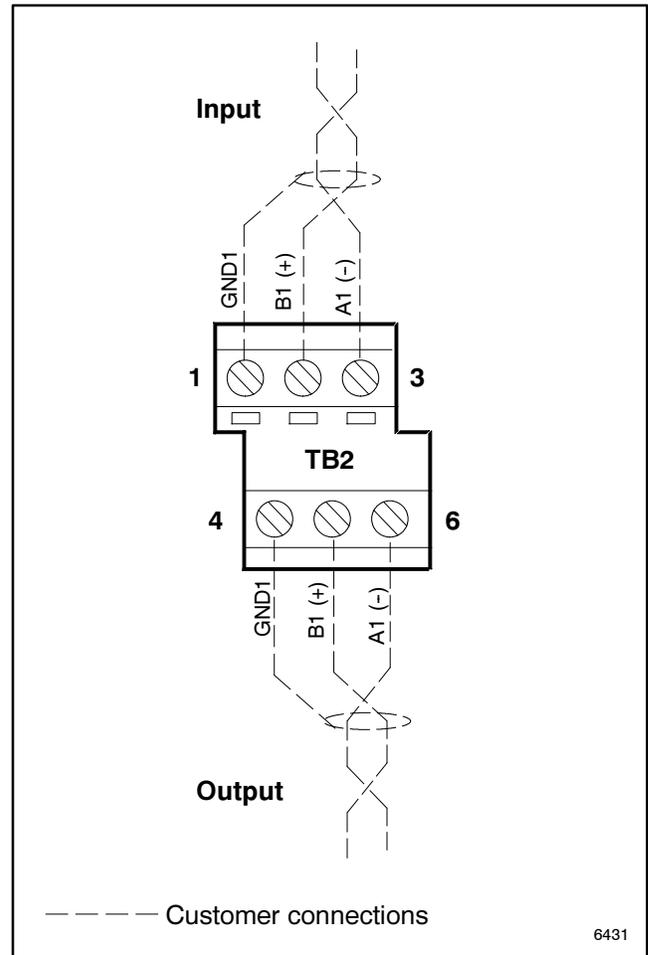
**Figure 6-3** Main Logic Board Modbus RS-485 Connections to TB2
