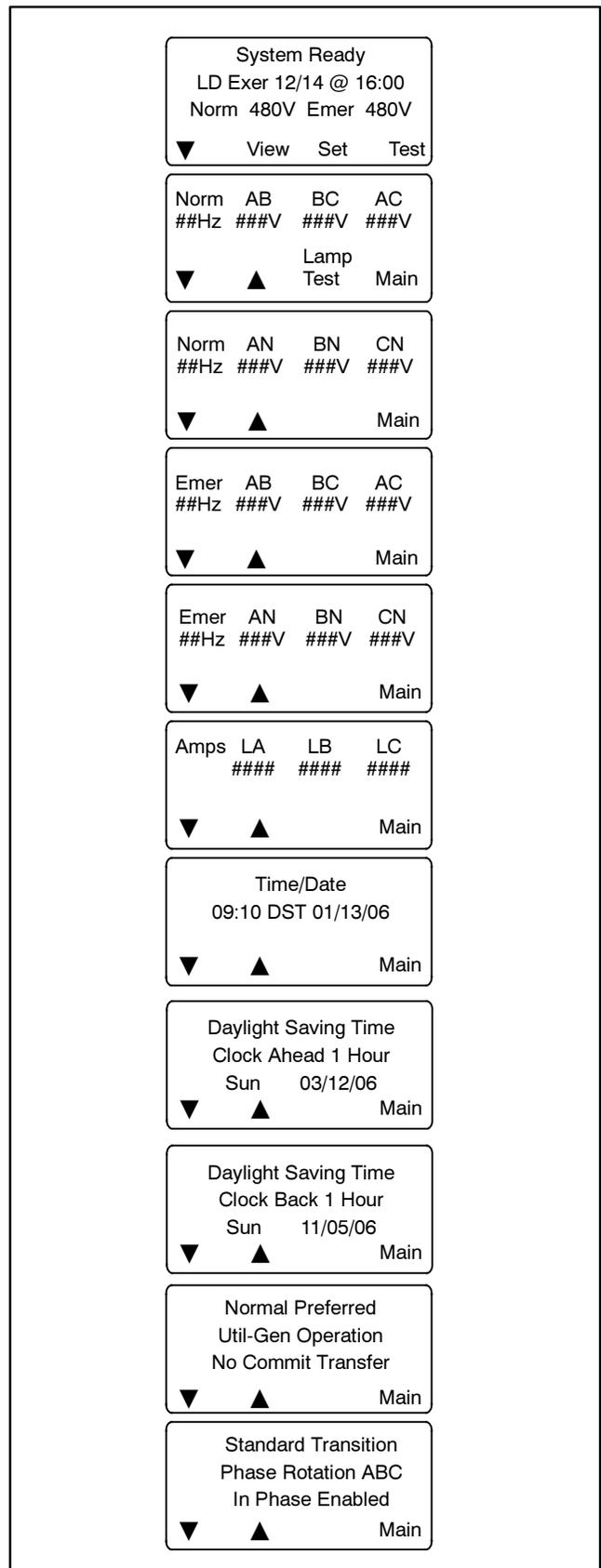
**Figure 3-10** Three-Phase Operation
