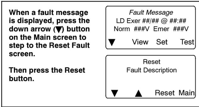
Figure 3-20 Fault Reset
