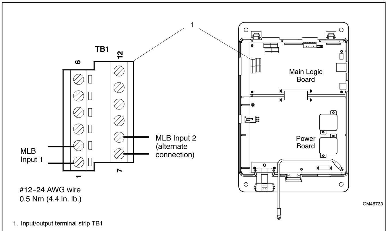
**Figure 8-24** Forced Transfer to Off Input Connection (for factory-installed load shed kits)
