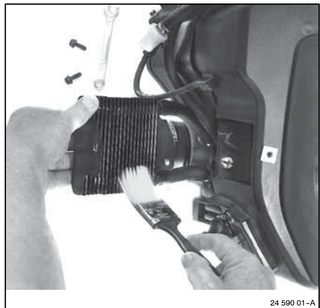
Figure 2-5 Cleaning the Oil Cooler
