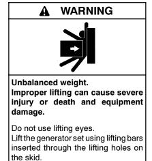
Approximate generator set weights are shown in Figure 1-1. Use lifting bars inserted through the holes in the skid to lift the unit. See the dimension drawings in Section 2 for lifting hole locations.
