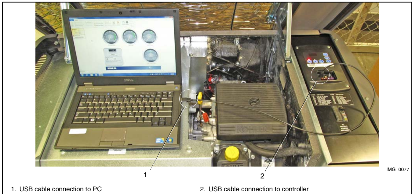
Figure 2-31 USB Connection for Firmware Update
