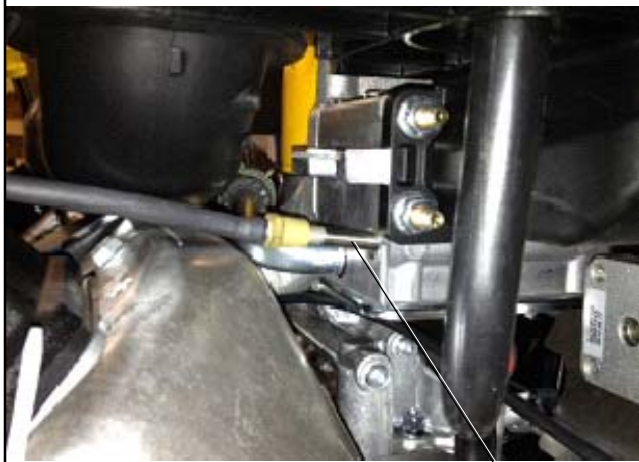
Figure 1-42 240 Volt Power Connection for Carburetor Heaters
