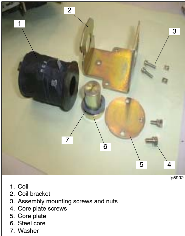
Figure 7-10 Coil Assembly Parts
