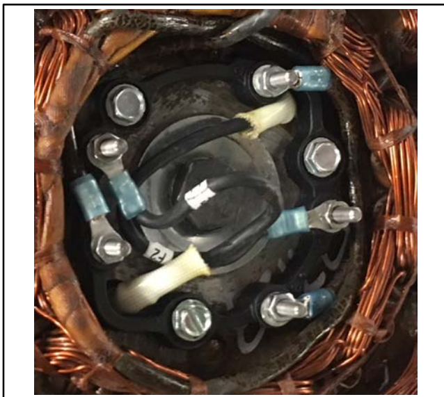
Figure 4-21 Disconnect Leads to Studs on Spacer
