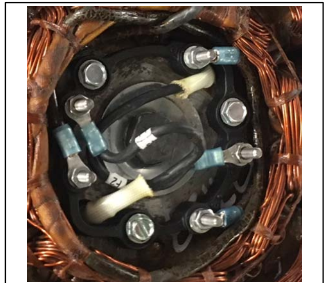
Figure 4-25 Connect Leads to Studs on Spacer
