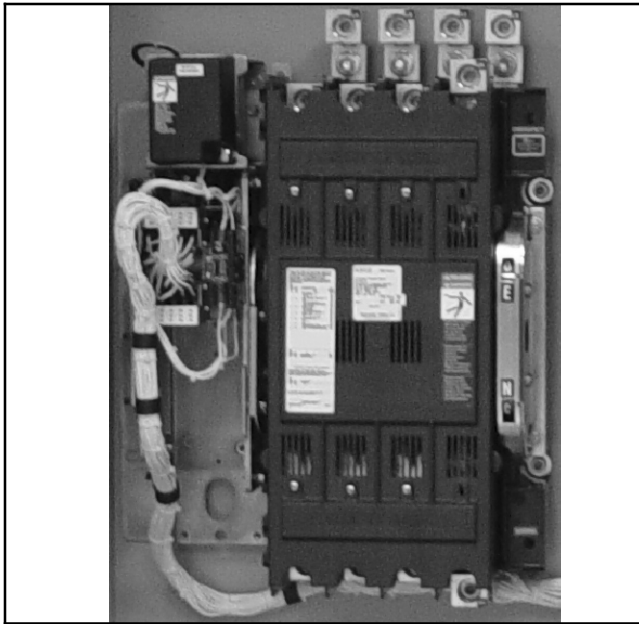
Figure 7-1 260- and 400-Amp Transfer Switches (3-pole with switched neutral shown, 260- and 400-amp have single-barrel terminal lugs)
