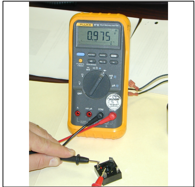
Figure 5-1 Checking Rectifier Diode Operation
