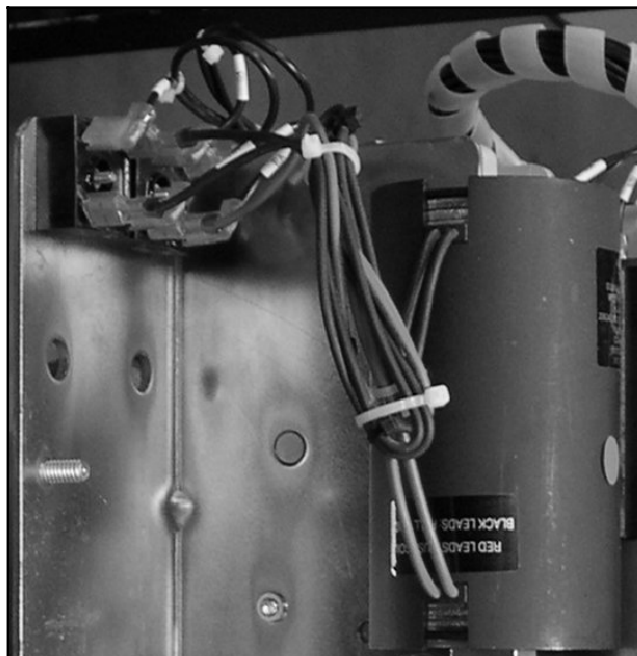
Figure 7-23 Rectifier Connections and Tie Wraps
