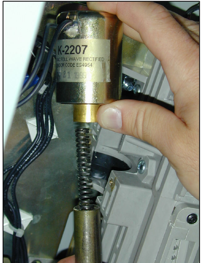
Figure 7-18 Spring and Plunger Assembly
