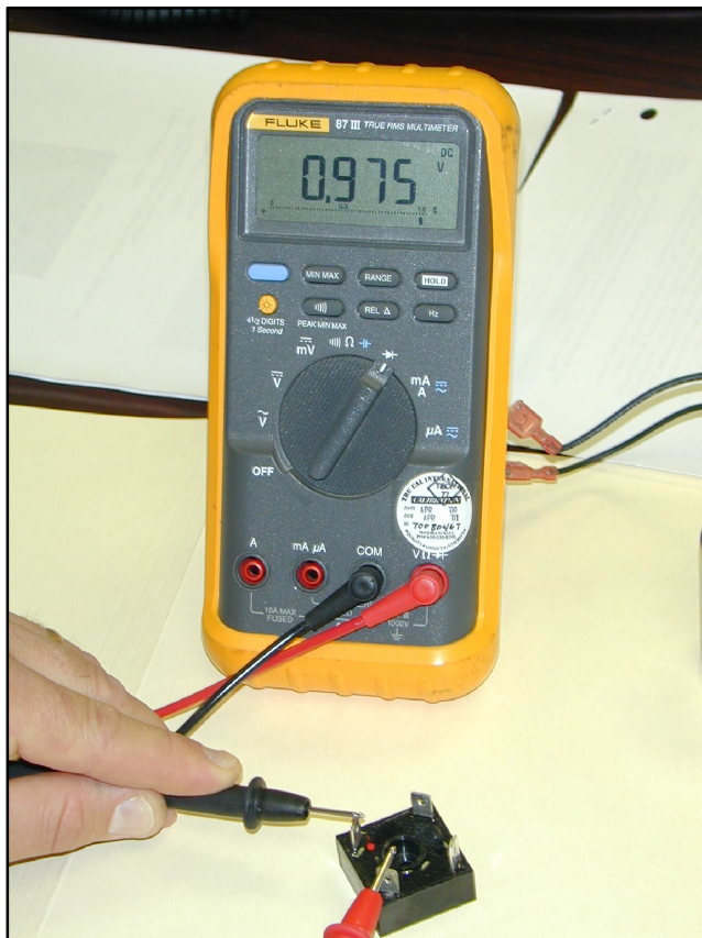
Figure 7-21 Checking Rectifier Diode Operation
