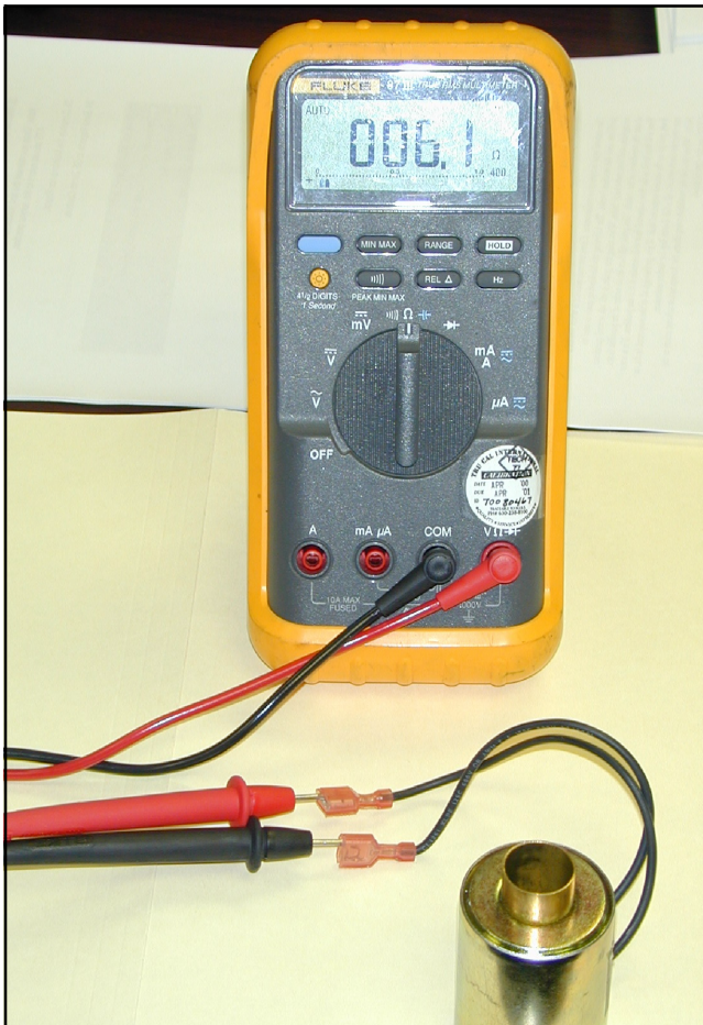
Figure 7-15 Checking Coil Resistance
