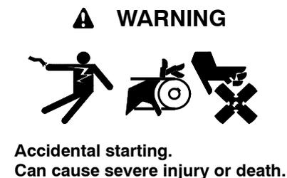
Disconnect the battery cables before working on the generator set. Remove the negative (-) lead first when disconnecting the battery. Reconnect the negative (-) lead last when reconnecting the battery.
