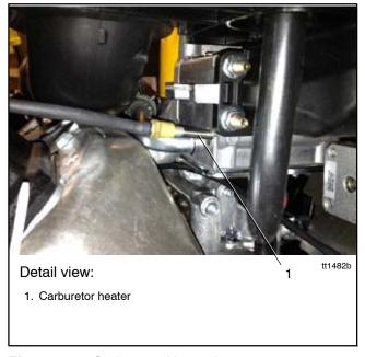
Figure 2-8 Carburetor Heater Location
