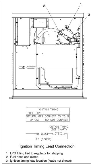
Figure 1-10 Fuel System, As Shipped
