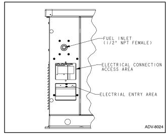
Figure 1-13 Electrical Connection Area
