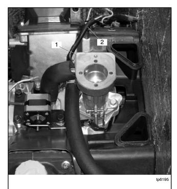
Carburetor heater (air cleaner removed to show heater)
