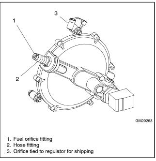
Figure 1-11 Fuel Orifice Fitting Installation
