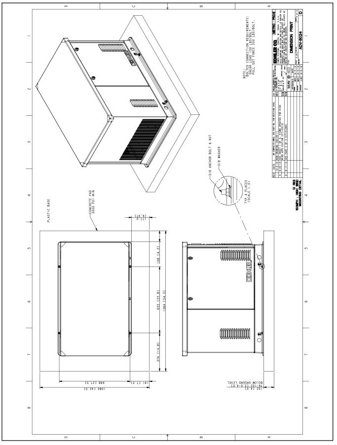
Figure 2-4 Dimension Drawing, ADV-8024, Sheet 3
