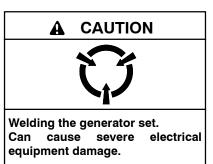
Never weld components of the generator set without first disconnecting the battery, controller wiring harness, and engine electronic control module (ECM).
