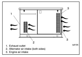
Figure 1-3 Cooling Air Intake and Exhaust, Typical
