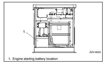
Figure 1-16 Battery Location, Air Intake End (typical)
