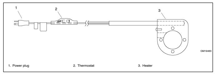
Figure 1-21 Carburetor Heaters
