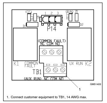
Figure 1-18 Relay Board Connections
