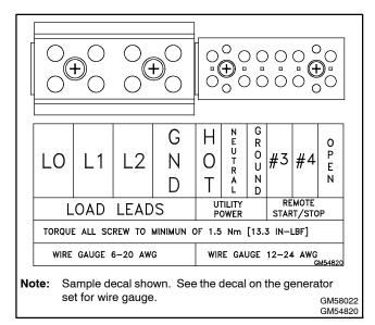
Figure 1-14 Field-Connection Terminal Block, typical
