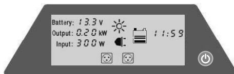
Figure 11 Simultaneous Charging and Output Mode with AC output
