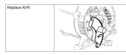
With engine stopped, replace AVR with a new AVR. Start engine and adjust trimmer on back of AVR. Test terminal voltage. Voltage should be between 95-135V. If voltage is met, original AVR is not adjusted properly or faulty. Replace as necessary. If voltage not met, check circuit breakers and receptacles.
