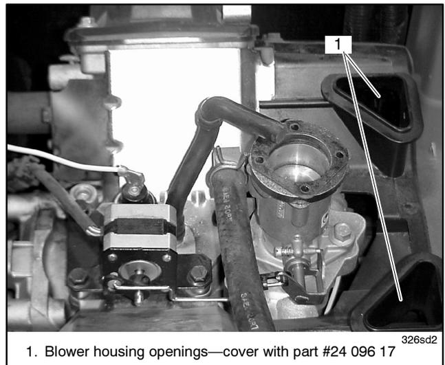
**Figure 6** Blower Housing Openings
