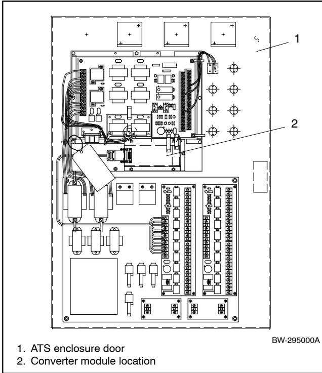
**Figure 4-11** Converter Module Location for M340/M340+ ATS Controllers
