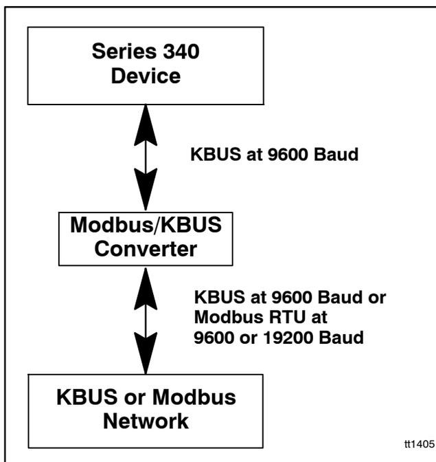
**Figure 4-1** Modbus/KBUS Converter Function
