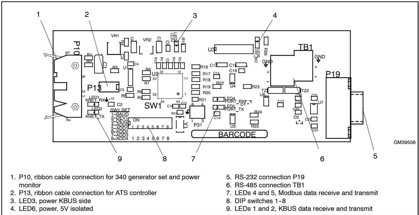
**Figure 4-2** Modbus/KBUS Converter Board
