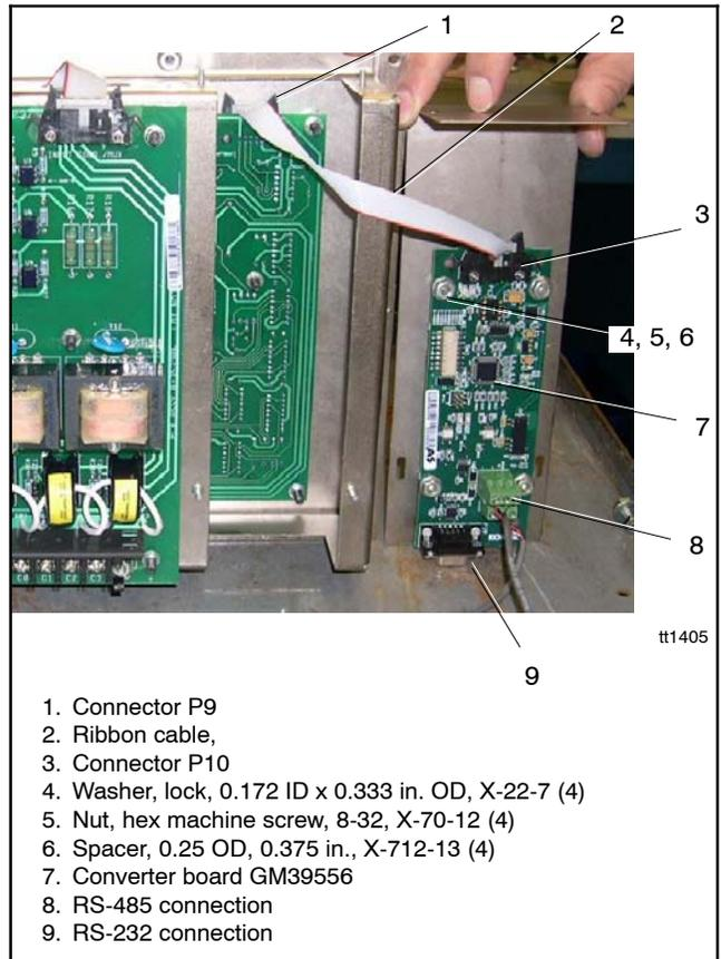
**Figure 4-16** Converter Module Installation Details for the Power Monitor
