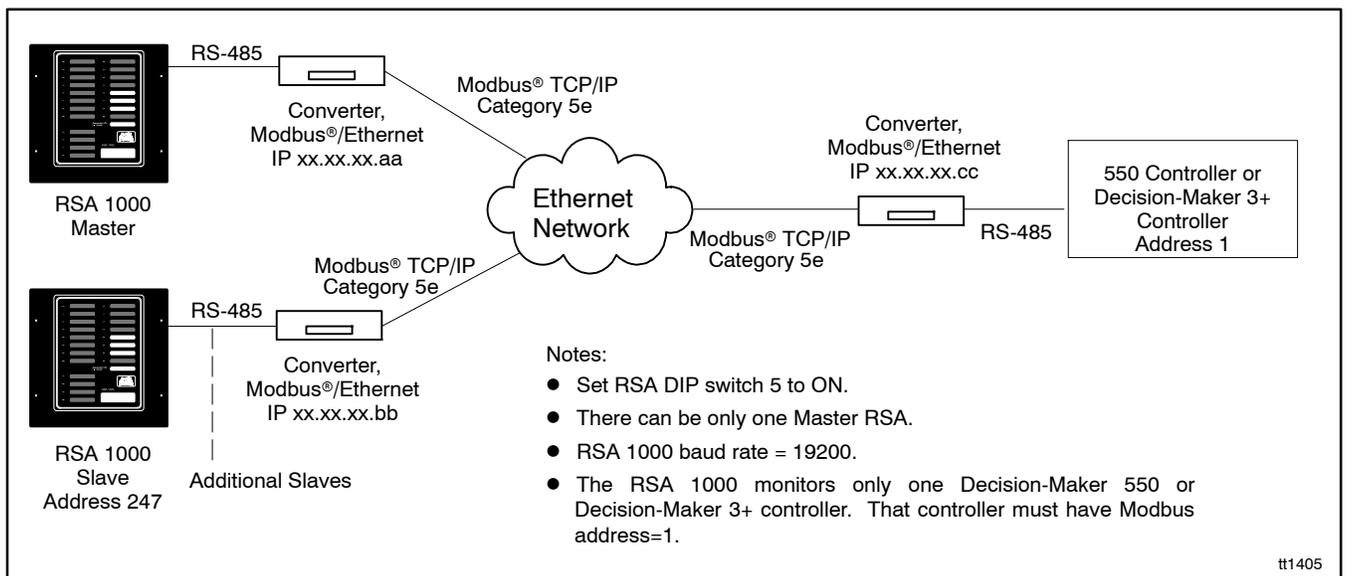
Figure 9-3 RSA 1000 Ethernet Network Connections
