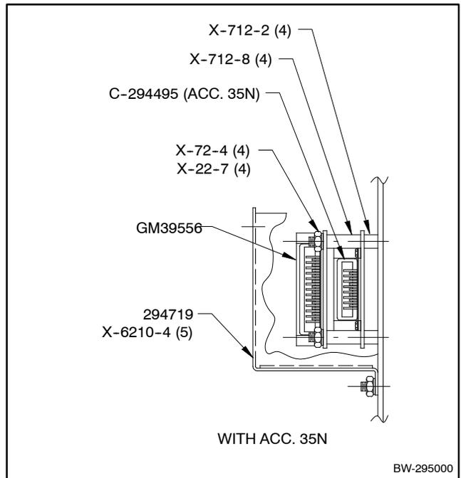
**Figure 4-14** Converter Module Installation Details for ATS Controllers With Load Shed Accessory 35N
