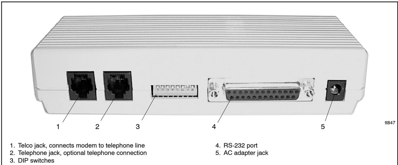
**Figure 3-5** External Modem (typical), Rear View
