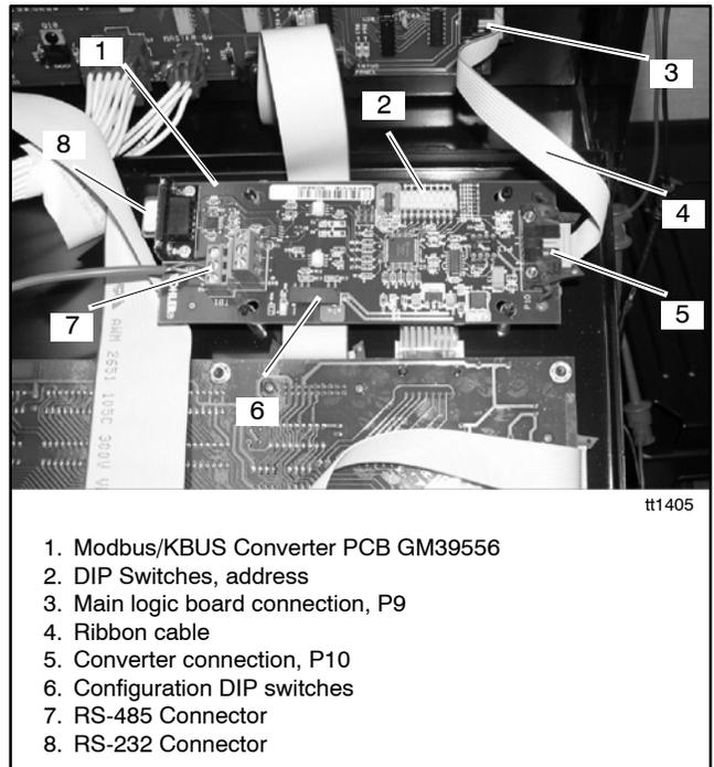
**Figure 4-10** Converter Connections and DIP Switches
