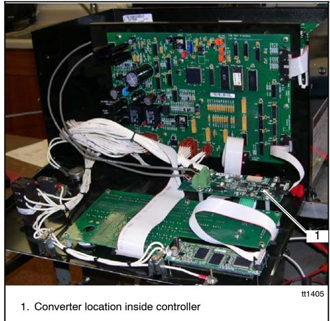
**Figure 4-9** Modbus/KBUS Converter Installation for the 340 Generator Set Controller
