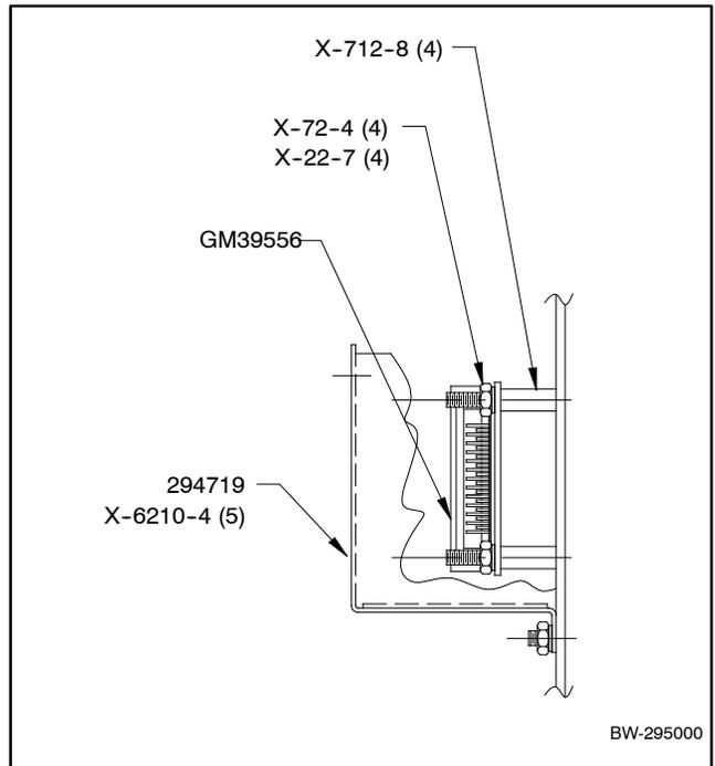
**Figure 4-13** Converter Module Installation Details for ATS Controllers Without Load Shed Accessory 35N
