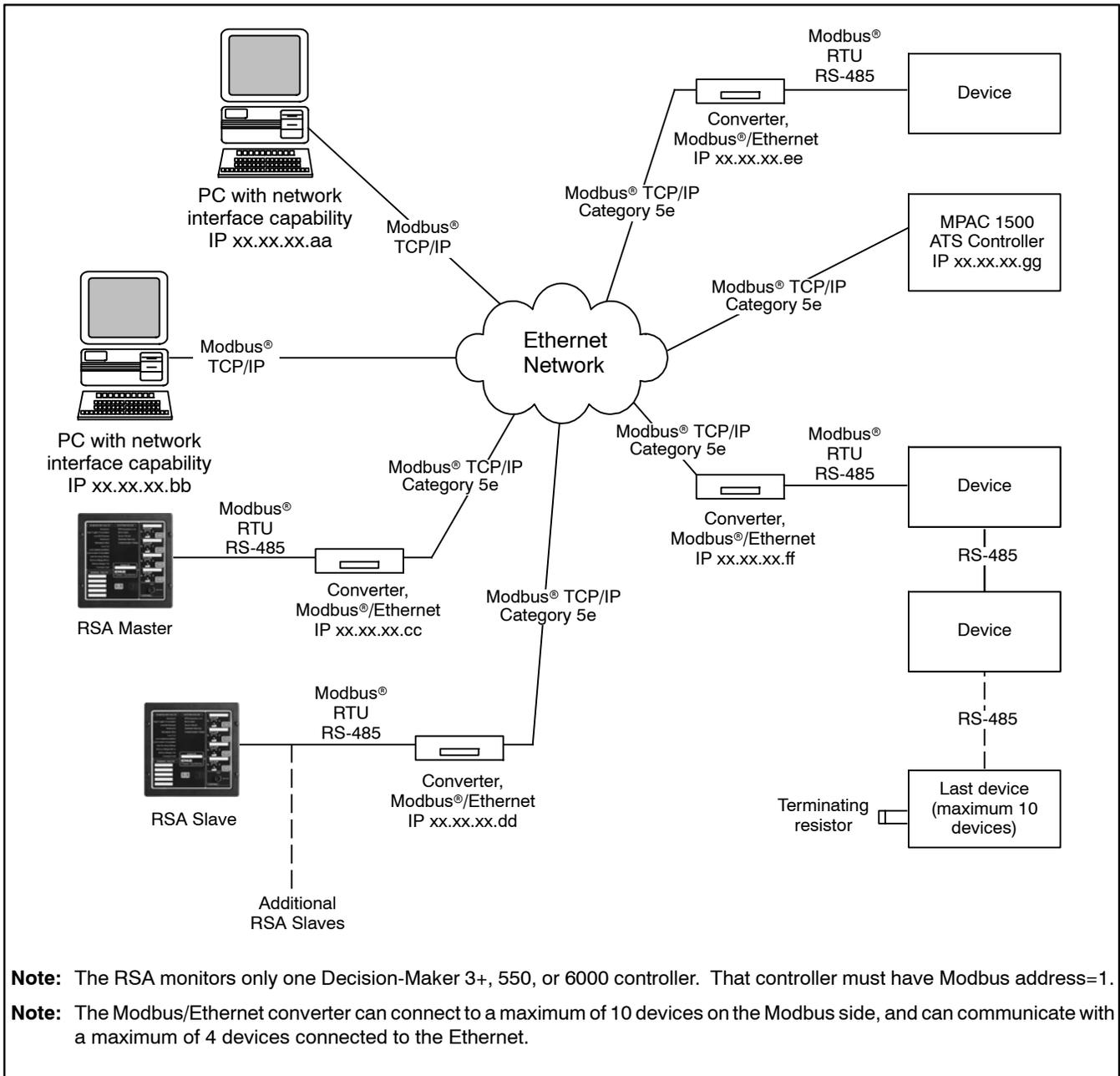
**Figure 2-3** Remote Network (Ethernet) Connection
