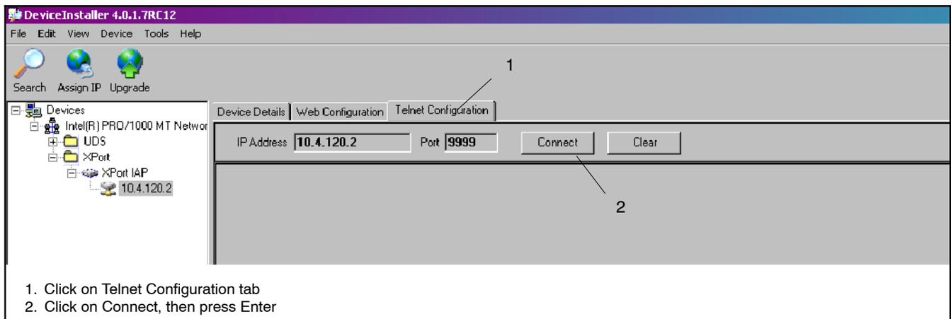
**Figure 14-15** DeviceInstaller Telnet Configuration Opening Screen
