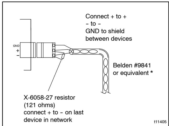
**Figure 7-2** RS-485 Connector Details
