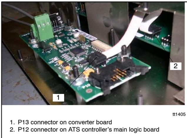
**Figure 4-12** Ribbon Cable Connection
