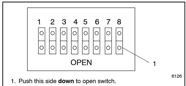
**Figure 5-5** DIP Switch Open Position
