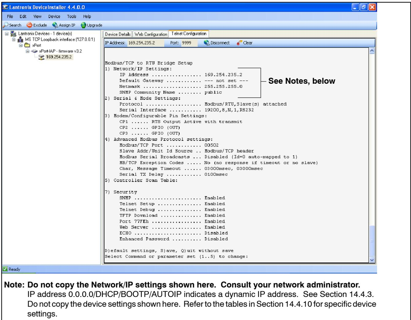
**Figure 14-16** Telnet Configuration Setup Mode Window for Controllers
