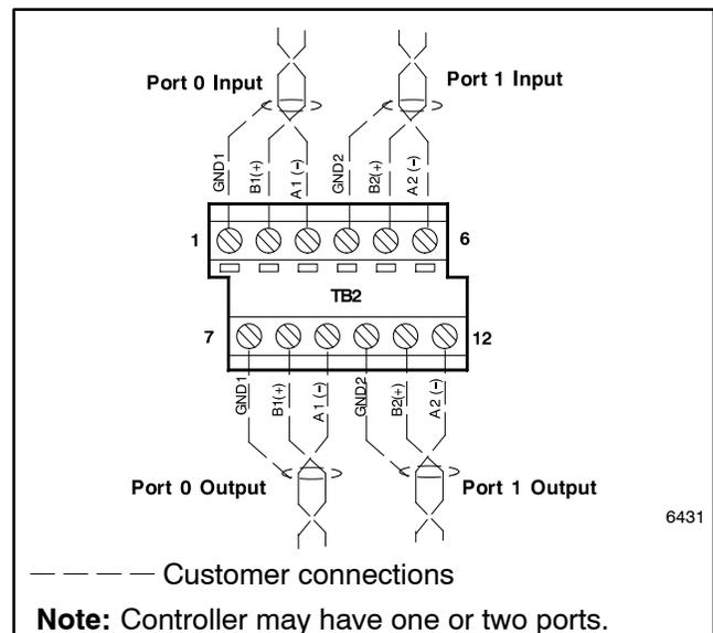
**Figure 12-2** Main Logic Board Modbus RS-485 Connections to TB2
