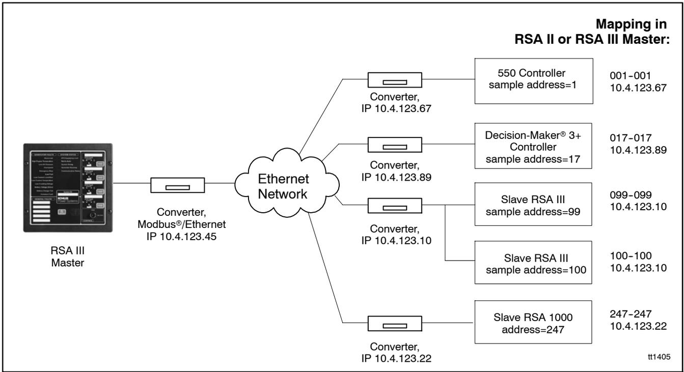
**Figure 14-24** RSA II or RSA III Connections with Sample Addresses and Mapping
