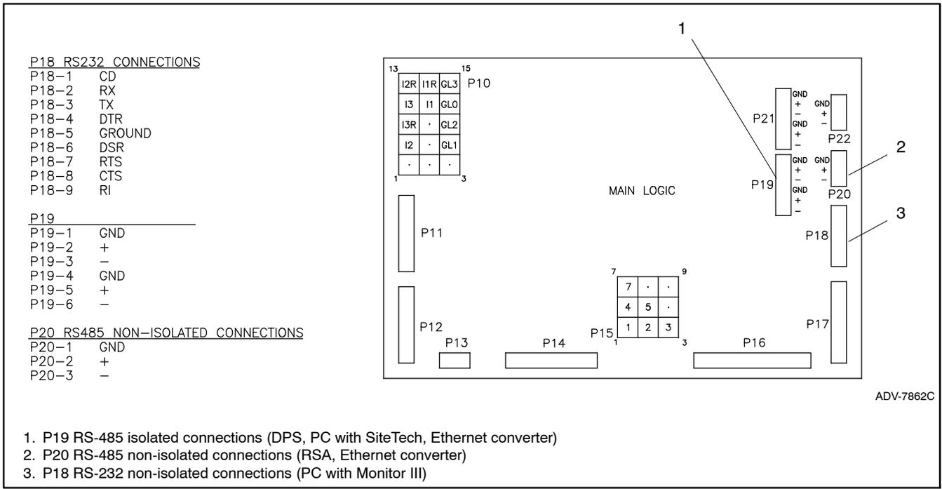
**Figure 7-3** Decision-Maker 6000 Controller Modbus Communication Ports
