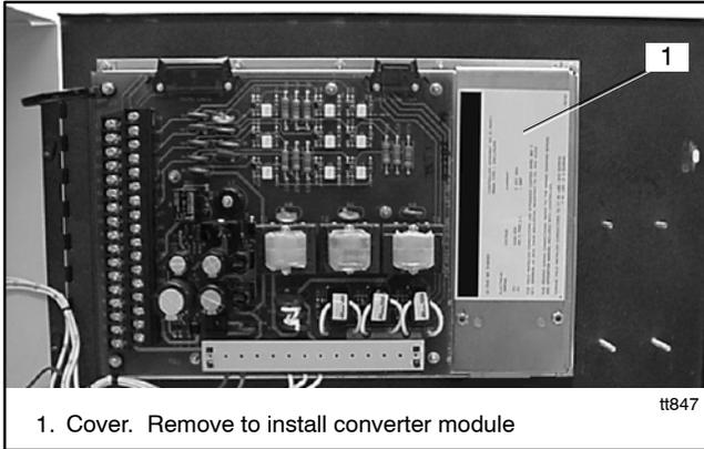
**Figure 4-15** Converter Module Location and Connection for the Power Monitor
