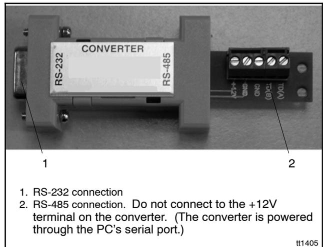
Figure 3-2 RS-232 to RS-485 Port Converter
