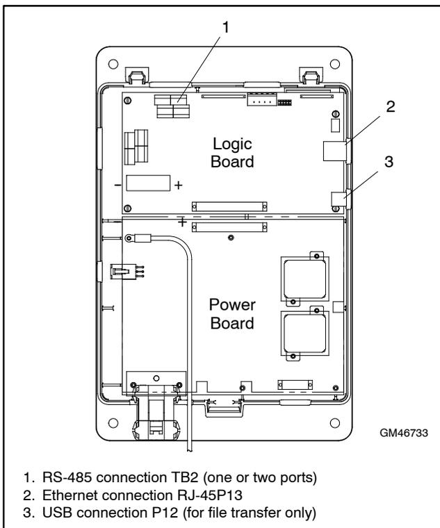
**Figure 12-1** Communication Connections (controller cover removed for illustration only)
