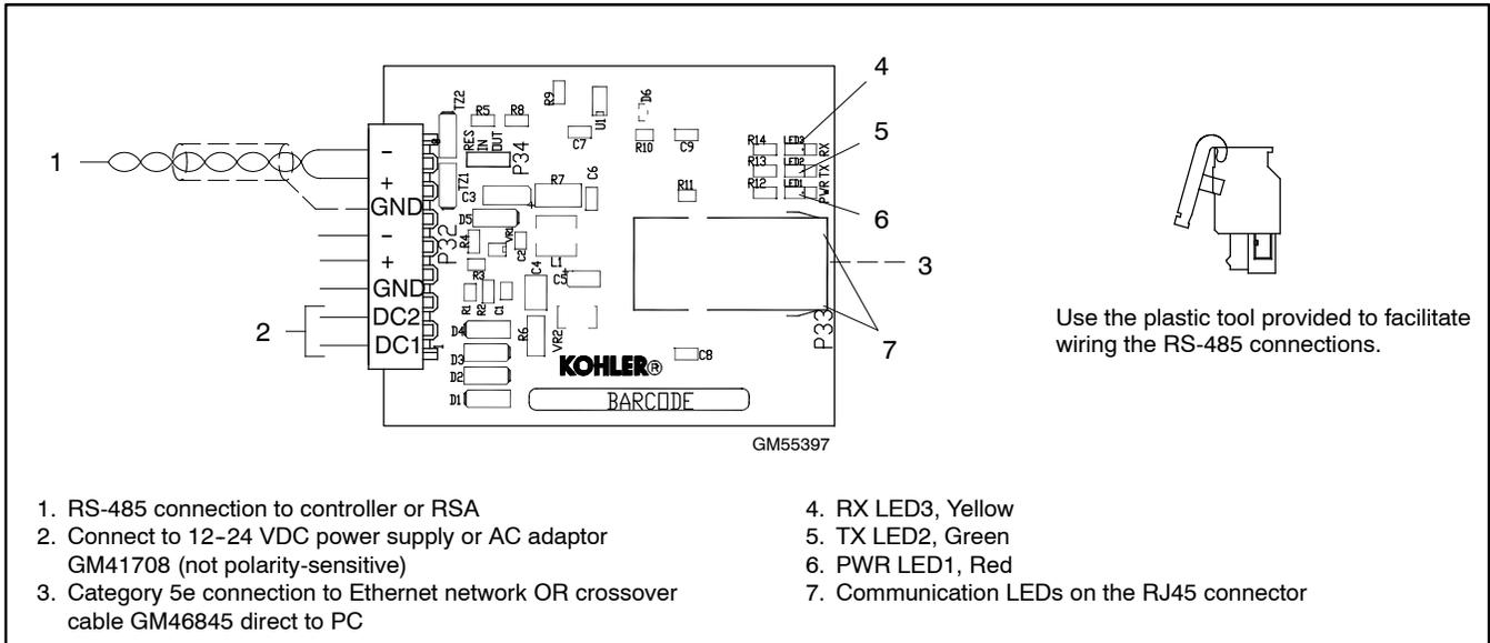
**Figure 14-3** Converter Connections
