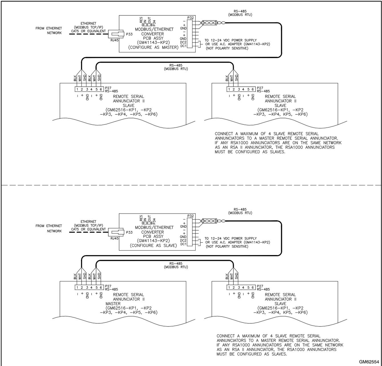
Figure 10-1 RSA II to Modbus/Ethernet Converter Connection Details
