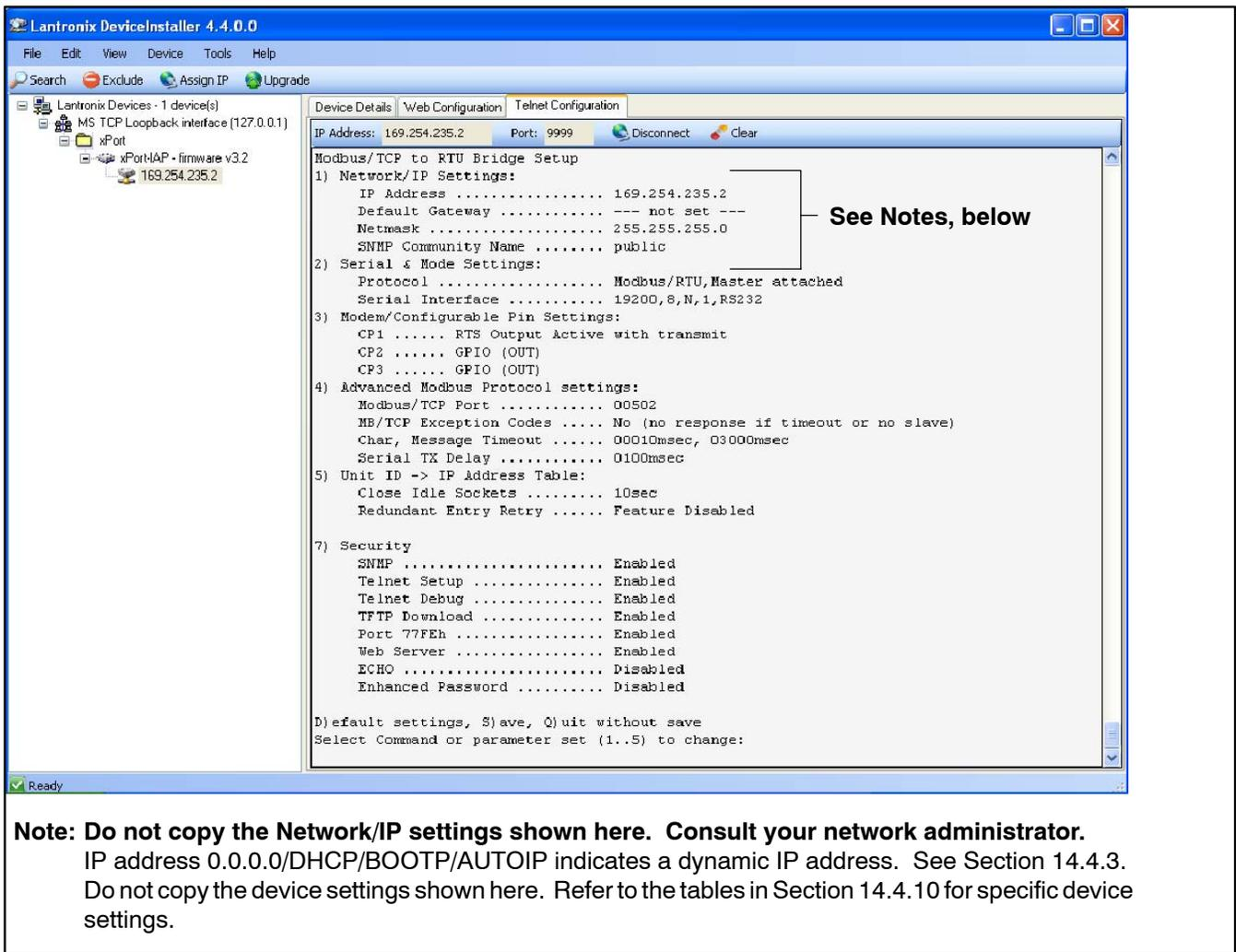
**Figure 14-17** Telnet Configuration Setup Mode Window for an RSA Master
