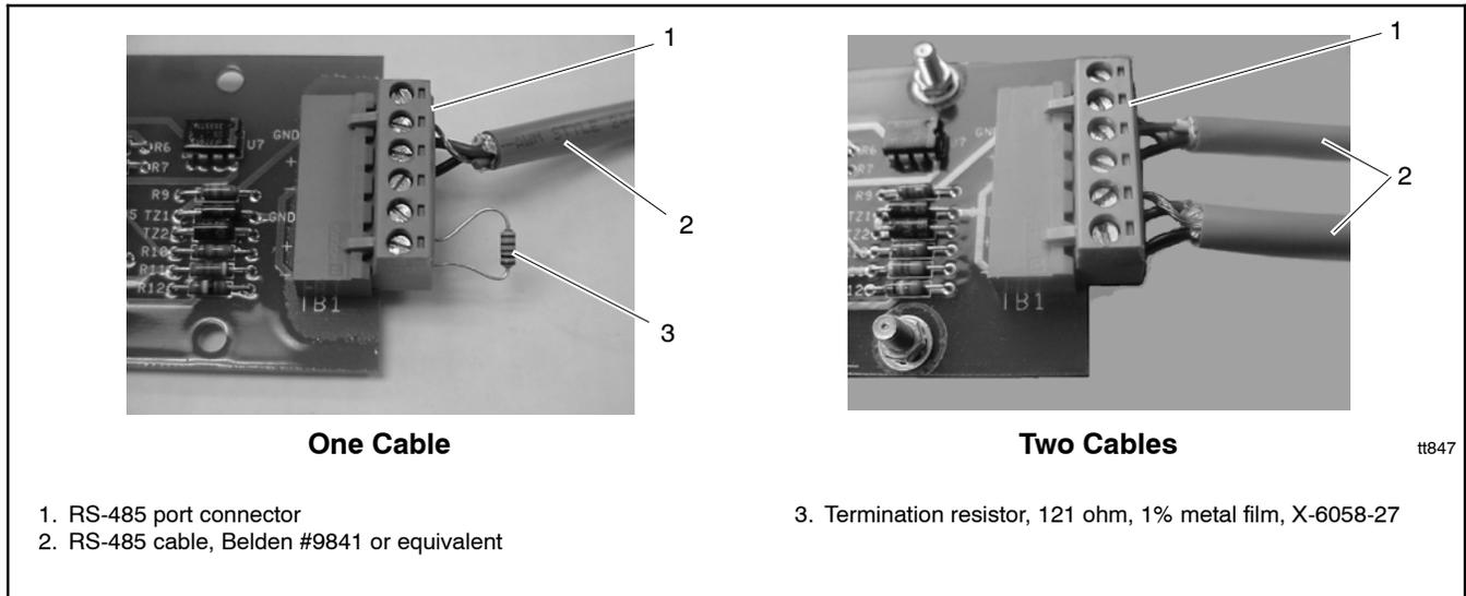
Figure 3-1 RS-485 Cable Connection Details
