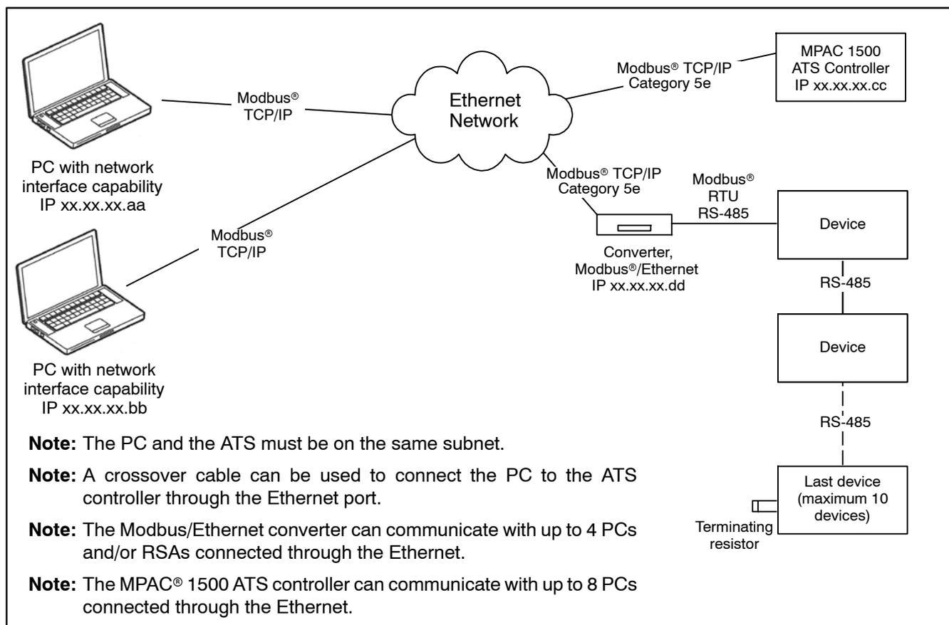
**Figure 12-3** Ethernet Connections to Multiple-Device Network
