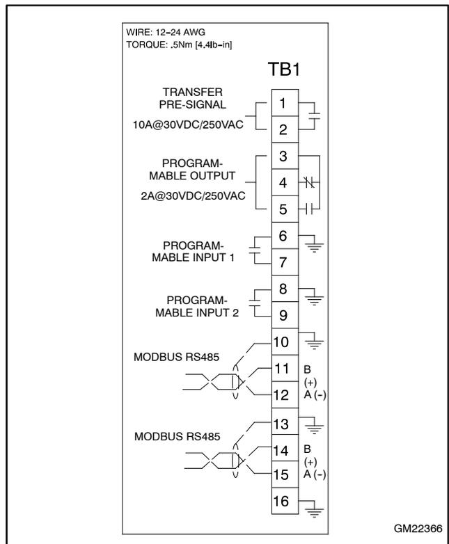
**Figure 11-2** Terminal Strip TB1 Connections
