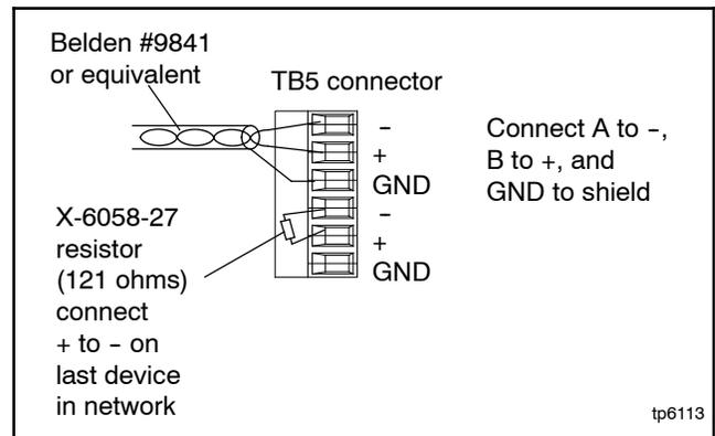
**Figure 5-3** RS-485 Connection Details
