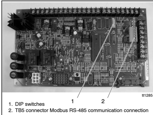
**Figure 5-1** Decision-Maker 3+ Controller Circuit Board GM28725 (red board)
