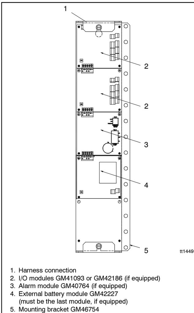
**Figure 13** Module Mounting Bracket with Modules
