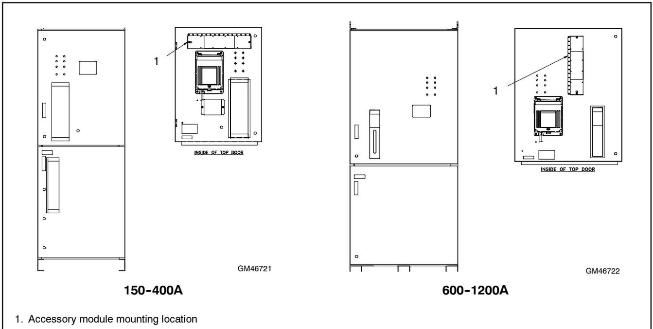
**Figure 9** Module Mounting Location, 150-1200A Model KG/SG Bypass/Isolation Switches
