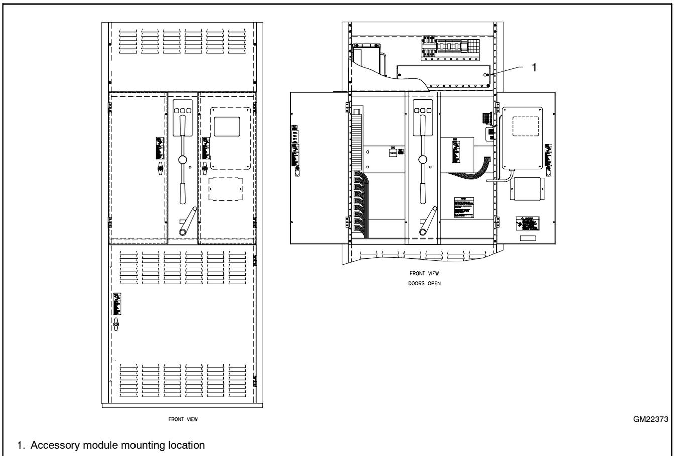
**Figure 10** Typical Module Mounting Location, 1600-3000A Model KB/SB Bypass/Isolation Switches
