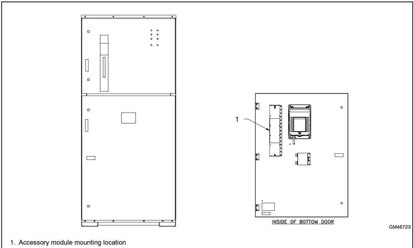
**Figure 11** Typical Module Mounting Location, 1600-3000A Model KG/SG Bypass/Isolation Switches
