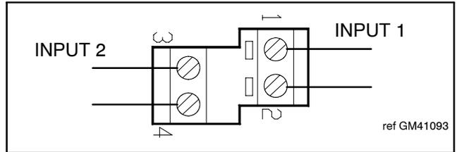
**Figure 17** I/O Module Input Connections (TB1 or TB10)
