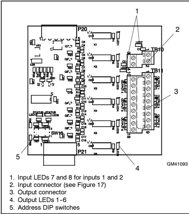
**Figure 15** Standard I/O Module GM41093
