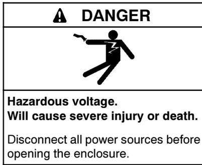
1. Disable the generator set and disconnect power to the transfer switch.
