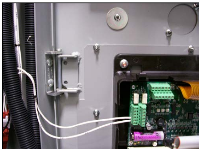
Figure 48 Connect Leads 20 and 33 to Programmable Input 1 on New Controller
