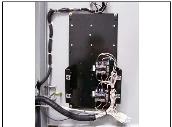
Figure 51 Upper Circuit Board Removed
