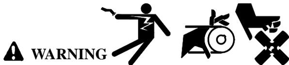
**Accidental starting can cause death or serious personal injury.** Turn Generator Master Switch to OFF position, disconnect power to battery charger, and remove battery cables (remove negative lead first and reconnect it last) to disable generator set before working on any equipment connected to generator. The generator set can be started by automatic transfer switch or remote start/stop switch unless these precautions are followed.
