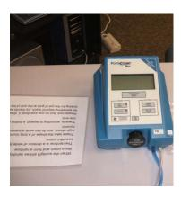
Provides accurate fit testing for PPE, SCBA, and Millenium masks.
