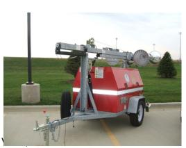
20 Kw diesel-powered with 4 – 1000 w floodlights.
