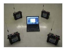
Monitors/Analyze air quality and travel distance of unknown "plume" of an hazardous material in and around an incident.
