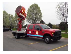
100 hp fan motor on elevating, rotating, and tilting stalk. Used for hi-rise ventilation, confined space ventilation, mass decontamination/cooling (with attachment for hose), toxic gas dissolution, etc.
