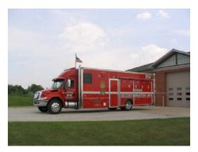
Capabilities: Mass decontamination – up to 200 people with supplies on board. Shower and hygiene facilities. Exterior, under-awning, misting nozzles for cooling.
