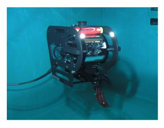
Remotely operated underwater high resolution imaging device, sonar helps locate and navigate to victims even in zero visibility; allows operator to manipulate interlocking saw to retrive victims or evidence.
