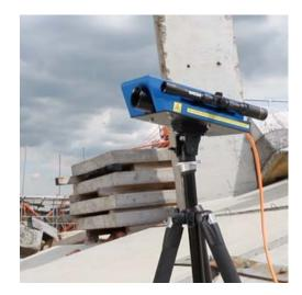
Lazer operated safety device that monitors building movement during Technical Rescue/Structural Collapse operations.
