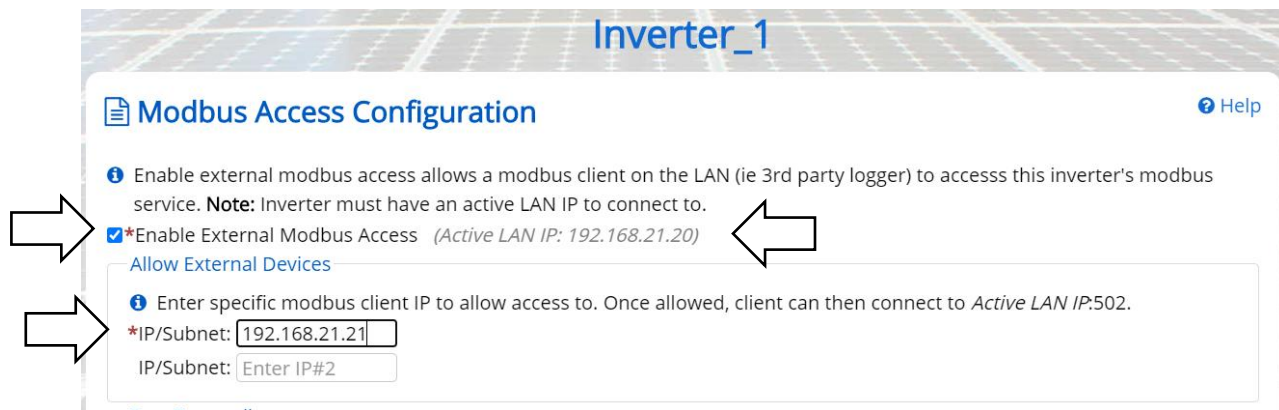
Figure 5-8 Enabling external Modbus access, static routing
