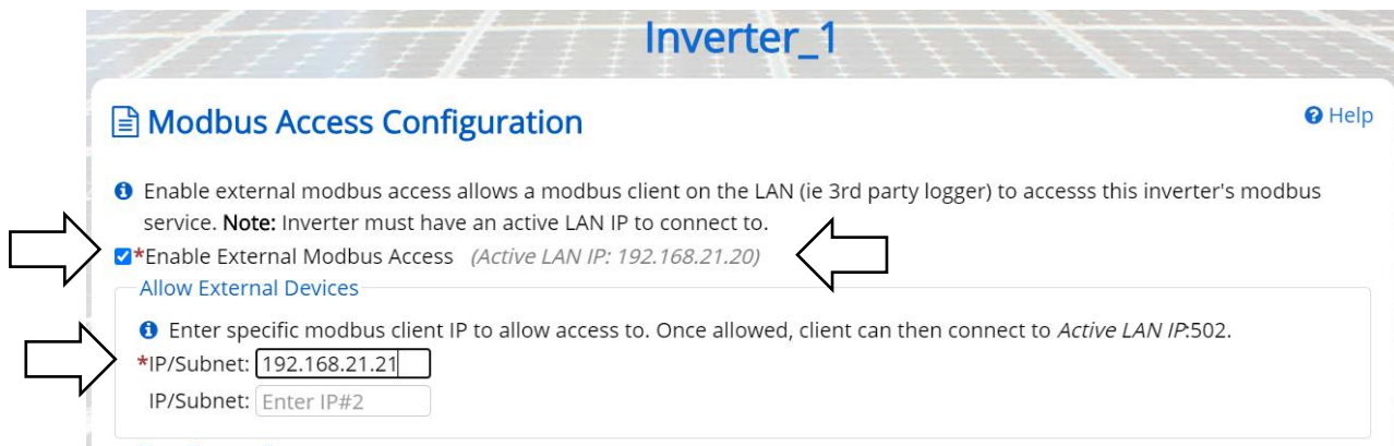
Figure 5-6 Enabling external Modbus access, Port Forwarding
