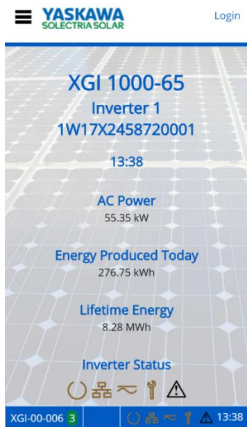
Figure 6-2 Inverter Home Page (Observer Mode)
