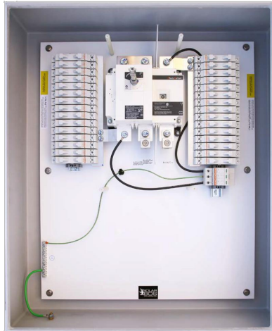
Floating Disconnect Combiner, 1500VDC, 275A disconnect, 15 input circuits, transient surge protection, NEMA-4X fiberglass enclosure
