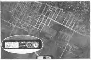
An aerial photograph taken with the new K-6 Automatic Recording Camera. The reproduction is about two-thirds full size. How the record made automatically on the bottom edge of the picture an indication of what record is shown in the center. On the left is the date, in the middle, the altitude at the time, below it, the focal length and lens number. At the bottom edge and finally the time record in hours, minutes and seconds. Next towards the right is the serial number of the camera.
